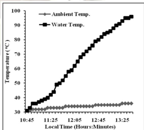
Figure 3: Temperature profiles of water and ambient condition during the full-load test.
