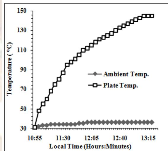
Figure 2: Temperature profiles of absorber plate and ambient condition during the stagnation test.
