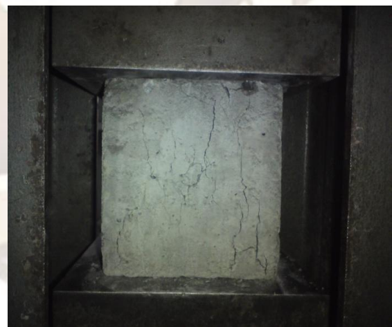
Fig No: 3- Failure of Cube at Ultimate Load
