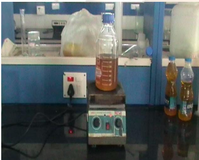
Fig:1.2. Transesterification process for Biodiesel
