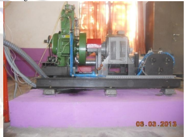
Fig: 2.1: Experimental Setup of eddy current dynamometer
