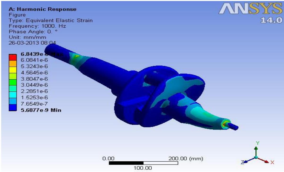
Figure 6, Equivalent Elastic Strain
