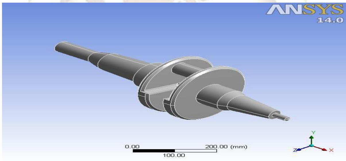
**Figure 1, Geometric model of crankshaft of single cylinder SI Engine**
