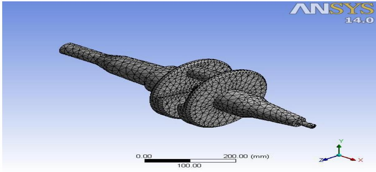
**Figure 2, FE Model of Crankshaft of Single Cylinder SI Engine**
