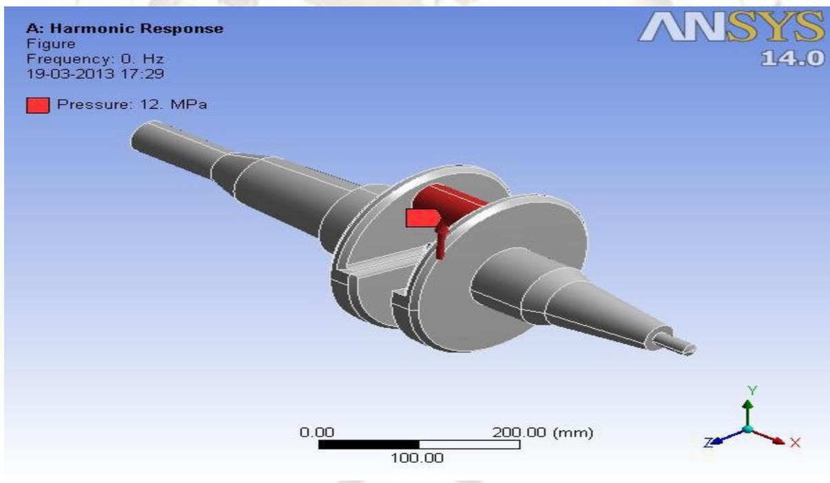
**Figure 3, Point of application of Pressure**
