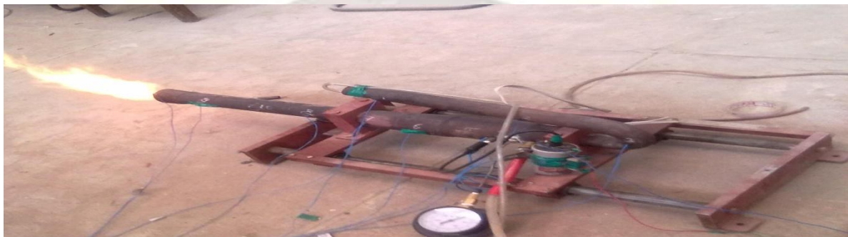
Fig.1.2: Experimental set up of 160 cm pulse jet engine2.
