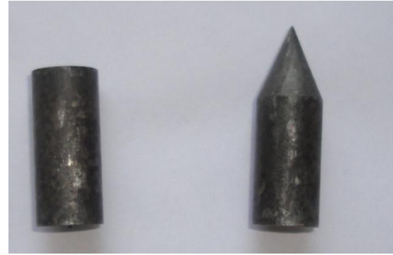
Fig. 2 The Blunt and Conical Nose Projectiles Used in the Study.
