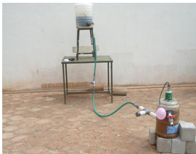
Fig-4 UASB Reactor after Production of Biogas
