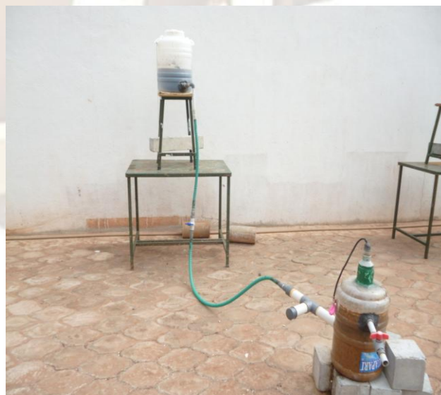
Fig-3 UASB Reactor before Production of Biogas
