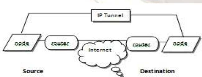
For end to end communication, we use IPSec modes. The two modes of IPSec are Transport Mode and Tunnel Mode. Transport mode is used to protect the protocol and Tunnel mode is used to protect the whole IP datagram. IPSec used to protects the voice and video traffic by tunnel. Here router works as firewall. The protocol used for voice is G.722 and for video is H.263. HMAC-MD5 used for data integrity mechanism.
