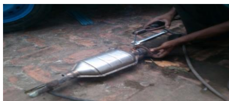
Fig 2: Catalytic converter to be welded in exhaust system of the car, Toyota E-90 in MIST welding shop.
