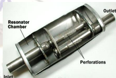
Fig 16: Muffler with built in resonator [6].
