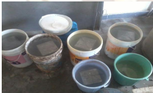
Fig 2: Curing of Cubes in sea water
