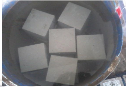
Fig 3: Curing of Cubes in H 2 SO 4 solution
