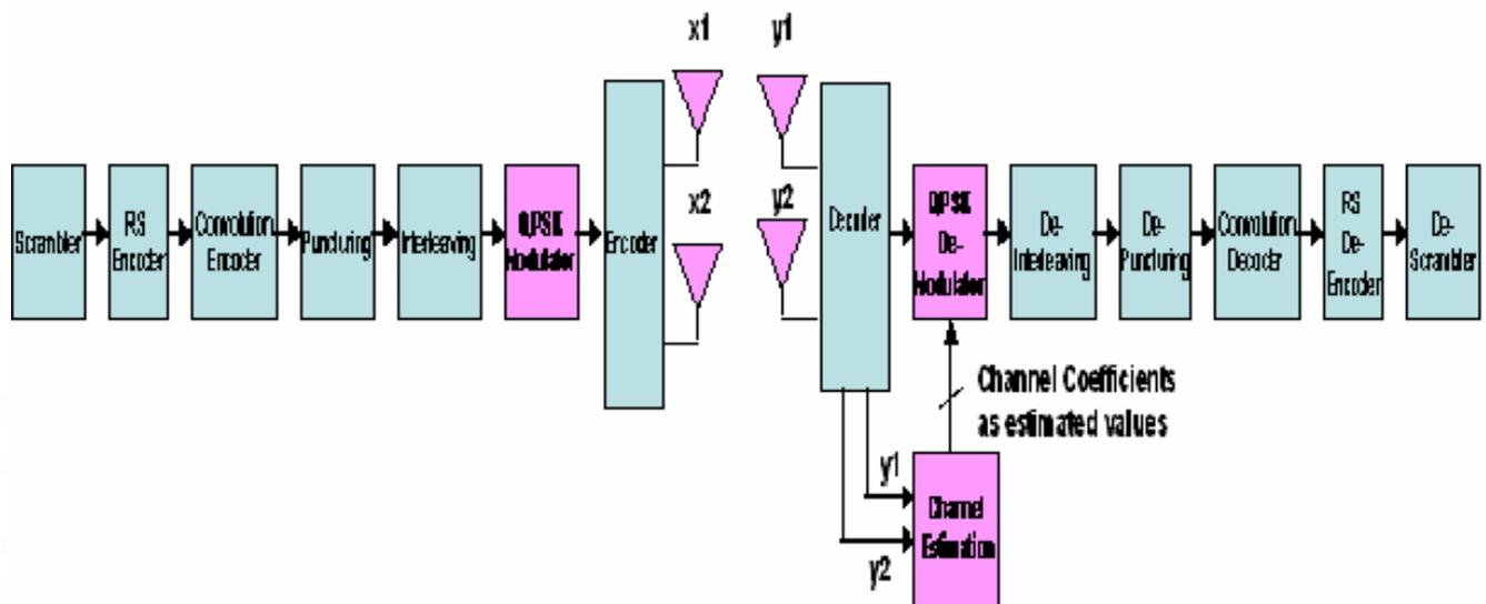
**FIG 3.1 Block Diagram of 8x8 MIMO system**
