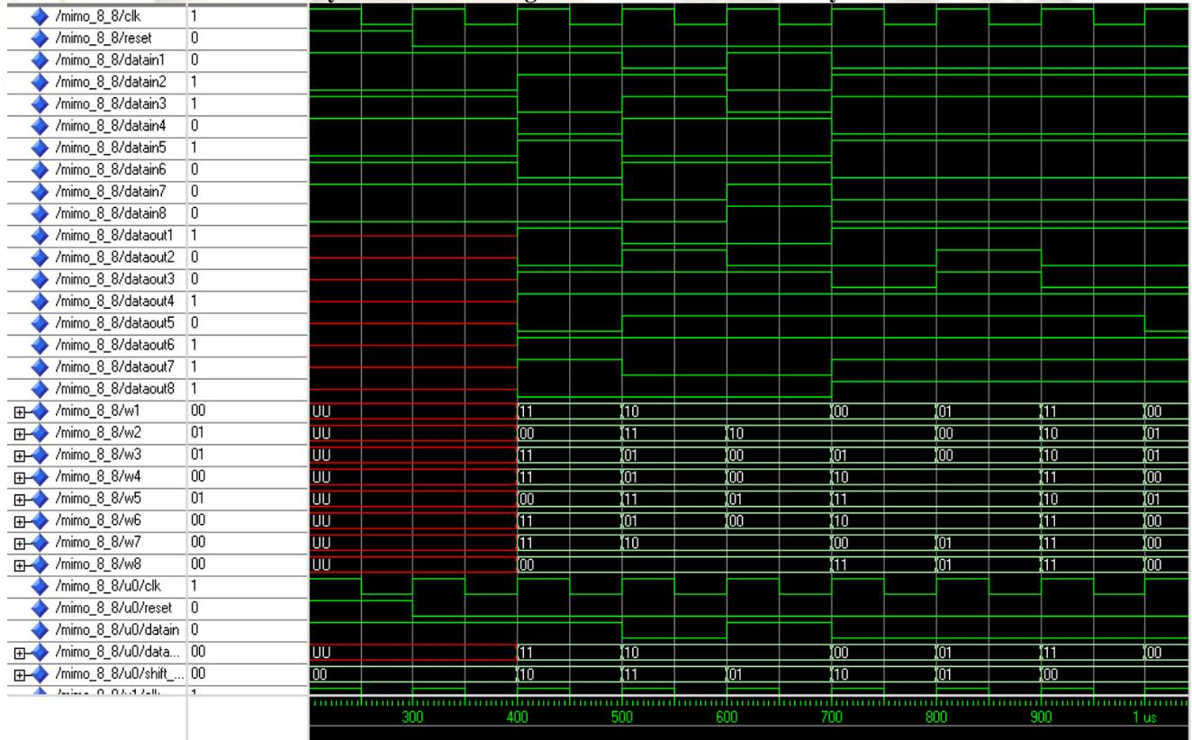
Fig.4.3 Output wave form of 8x8 MIMO using convolutional code
