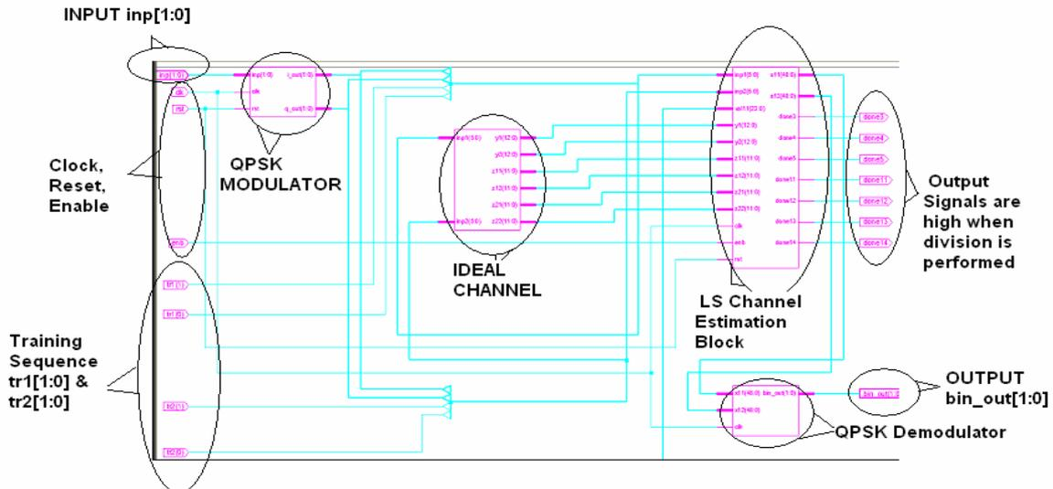
**FIG 4.1 MIMO System with QPSK Design**
