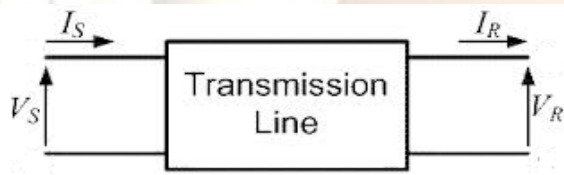
Fig 8. Two port model of a transmission line.
