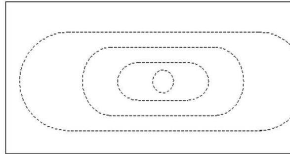
Fig. 14: Scan strategy to laser form the saddle shape, 800W , 20mm/s [3]
