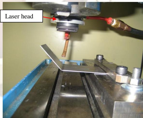
Fig. 2. Typical experimental setup of laser bending of metal sheet.[9]
