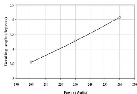
Fig.6. - Effect of laser power on the bending angle. Material: AISI1010, laser input power =200 – 260W, laser beam diameter = 2 – 3 mm, scan velocity = 2 – 4 mm/s, pulse duration = 7 – 11 ms [9]
