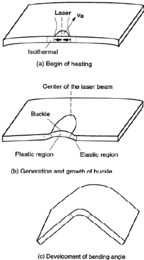
Fig 4. - The Buckling Mechanism[9]
