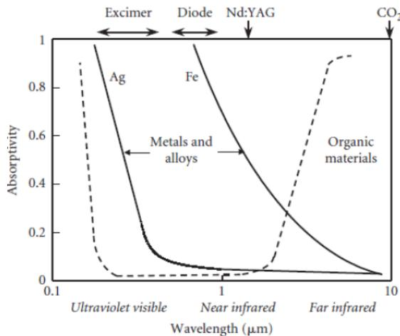
Fig.10 – Schematic of variation of absorptivity with wavelength for metals, alloys and organic materials .[9]
