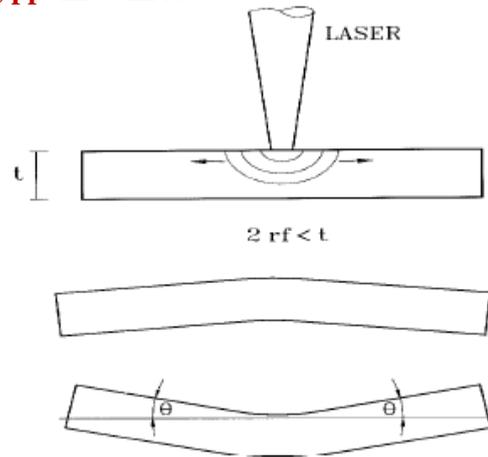
Fig. 3 Sequence of Temperature Gradient Mechanism[9]
