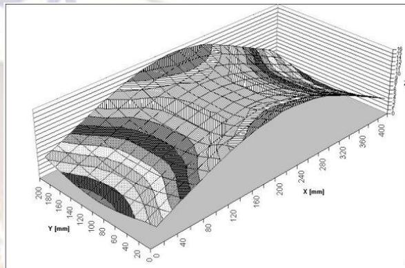
Fig. 15 3-D Contour plot of laser formed saddle shape[3].
