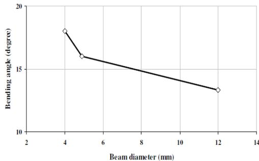
Fig.7- Effect of beam diameter on the bending angle . Process parameters; Material: AISI1010, laser input power =200 – 260W, scan velocity = 2 – 4 mm/s, pulse duration = 7 – 11 ms[9]
