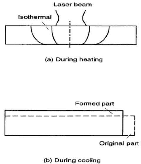
Fig.5 The upsetting mechanism[9]
