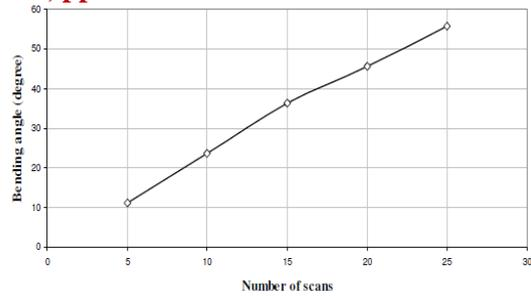
Fig .9 - Relationship between bending angle and number of scans. Process parameters: Material = Low carbon steel, laser input power = 170 W, laser beam diameter = 1.2 mm, scan velocity = 3 mm/sec, workpiece thickness = 1.2 mm[9]
