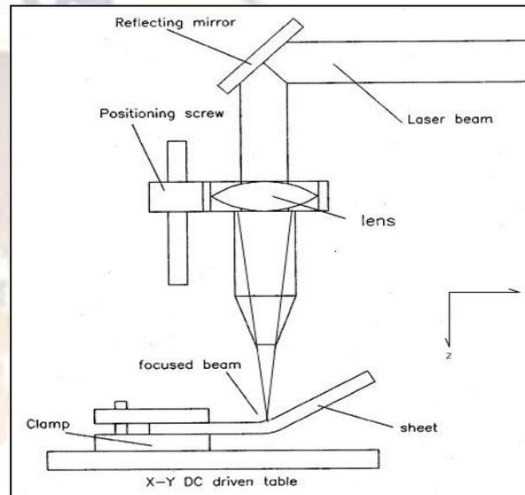
FIGURE 1: Simple Line diagram of Laser bending set up
