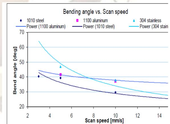
Fig.12 2θ-scan speed results for three different materials at 80 W after 15 scans[2].
