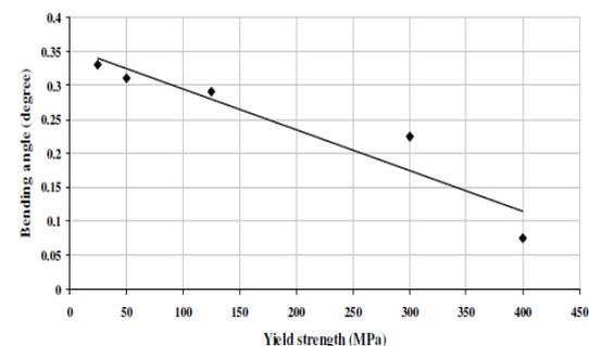
Fig.10 - Relationship between material yield strength and bending angle in degrees.[9]
