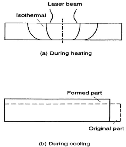
Fig.5 The upsetting mechanism[9]
