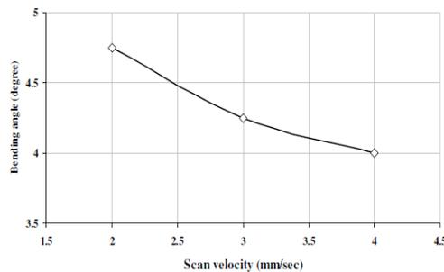
Fig.8 - Effect of scan velocity on the bending angle . Process parameters; Material: AISI1010, laser input power =200 – 260W, laser beam diameter = 2 – 3 mm, scan velocity = 2 – 4 mm/s, pulse duration = 7 – 11 ms[9]
