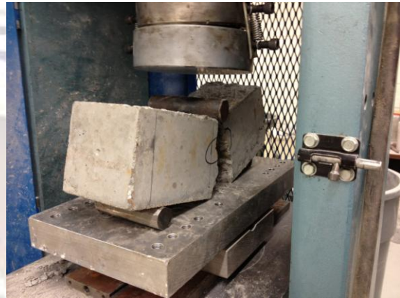
Figure 8: Typical beam failure, by flexure.
