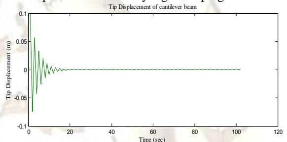
Fig. 7 The effect of negative velocity gain on the beam subjected to third mode vibration. (Gain=-1 V/A)
