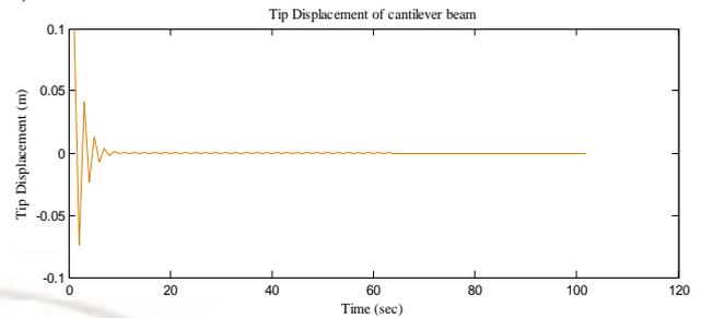
Fig. 6 The effect of negative velocity gain on the beam subjected to second mode vibration. (Gain=-5 V/A)
