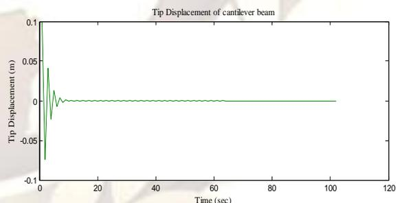
Fig. 8 The effect of negative velocity gain on the beam subjected to third mode vibration. (Gain=-5 V/A)
