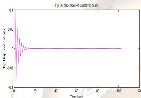
Fig. 3 The effect of negative velocity gain on the beam subjected to first mode vibration. (Gain=-2 V/A)
