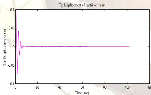
Fig. 4 The effect of negative velocity gain on the beam subjected to first mode vibration. (Gain=-5 V/A)
