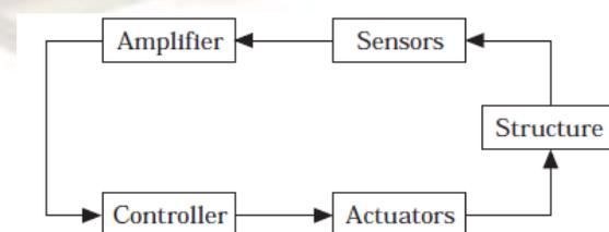
Fig.1 Block diagram of feedback control system
