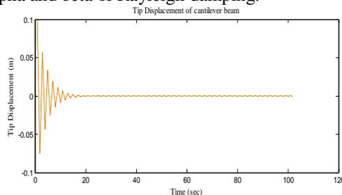
Fig. 5 The effect of negative velocity gain on the beam subjected to second mode vibration. (Gain=-1 V/A)
