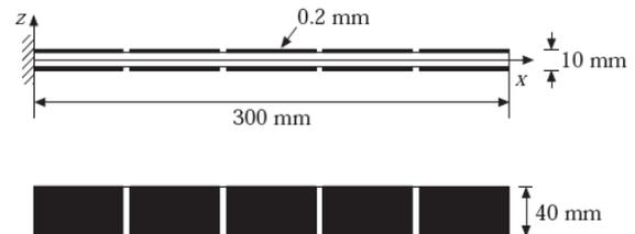
Fig. 2 A cantilever composite beam
