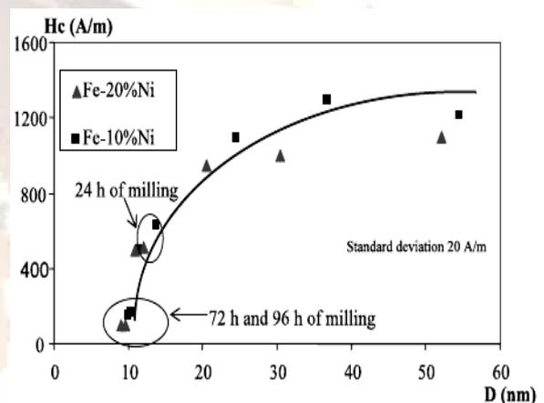
Fig 2 (b). The coercivity as a function of crystallite size
