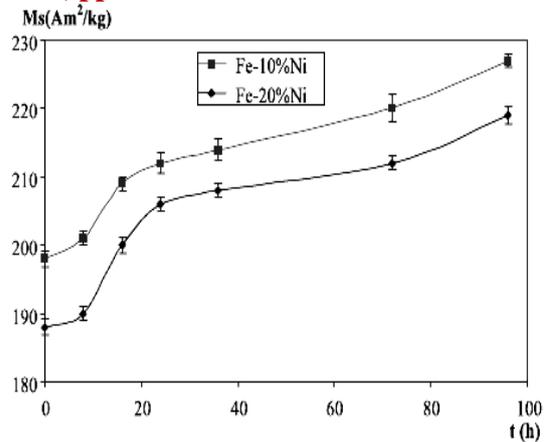
Fig 2 (a). Evolution of saturation magnetization versus milling time
