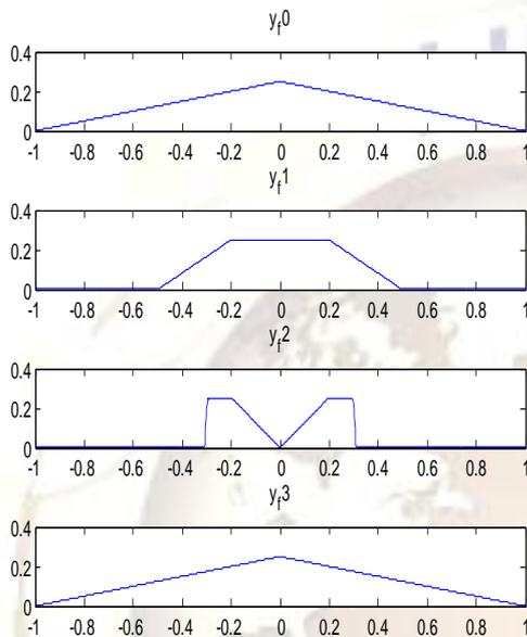
Fig. 4: Reconstructed output for four channel TMUX
