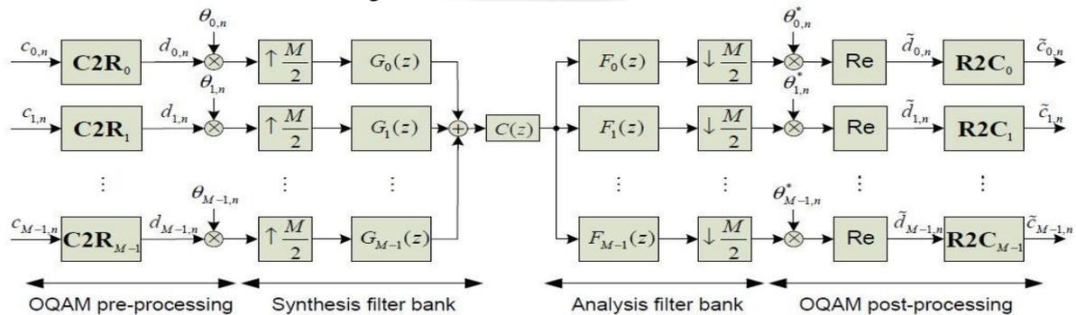
Fig. 2: Partial TMUX structure
