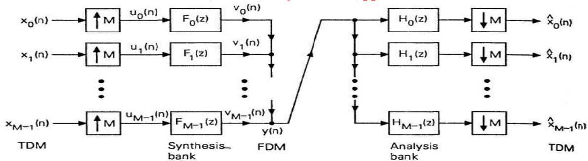
Fig. 1: General TMUX structure.
