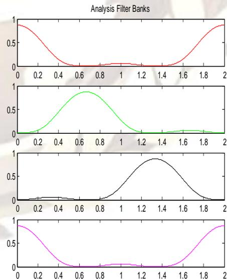
Fig. 6: Analysis Filter bank for Non-Maximally Decimated TMUX
