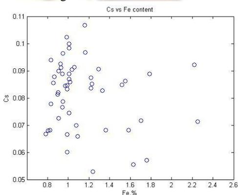
Fig 10. Sulphide capacity as a function of Fe content in slag
