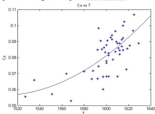
Fig 9. Sulphide capacity as a function of Temperature
