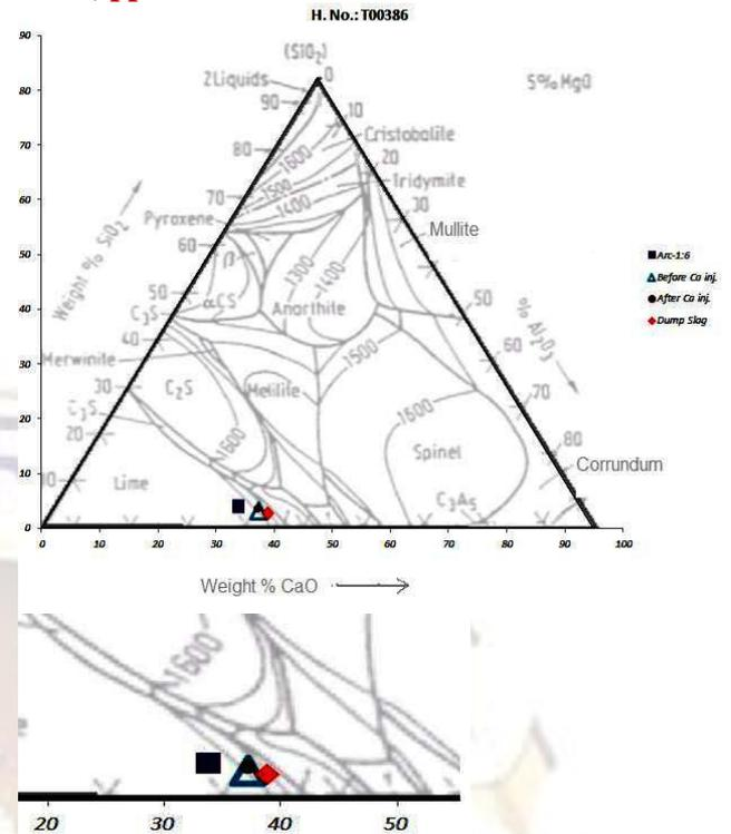
Fig3. Ternary diagram for CaO, Al<sub>2</sub>O<sub>3</sub>, SiO<sub>2</sub> system at constant 5% MgO for correlation with sulphide capacity (having low C<sub>s</sub>)
