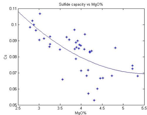
Fig 6. Sulphide capacity as a function of saturated MgO. It shows that for better desulfurization reaction rate, it will be very effective to decrease the MgO content. Likely effect on increasing viscosity
