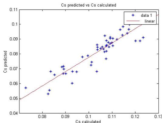
Fig 11. Sulphide capacity predicted as a function of Sulphide Capacity calculated
