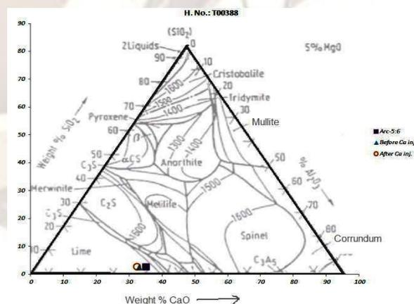
Fig1. Ternary diagram for CaO, Al<sub>2</sub>O<sub>3</sub>, SiO<sub>2</sub> system at constant 5% MgO
