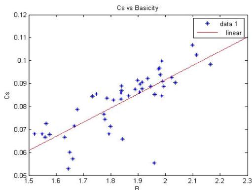
Fig 8. Sulphide Capacity values as a function of Basicity
