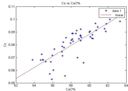
Fig 5. Sulphide Capacity as a function of CaO content of slag
