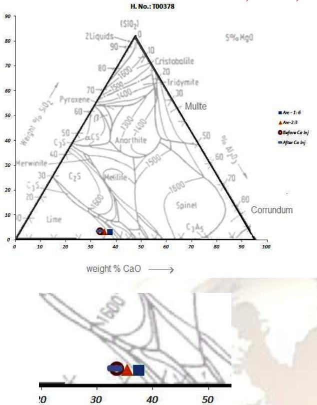
Fig4. Ternary diagram for CaO, Al<sub>2</sub>O<sub>3</sub>, SiO<sub>2</sub> system at constant 5% MgO for correlation with sulphide capacity
