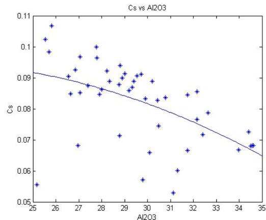
Fig 7. Sulphide Capacity as a function of Alumina in slag
