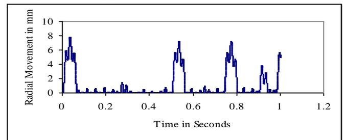
Fig.10 Cu particle radial movement for 220kV with FEM electric field
