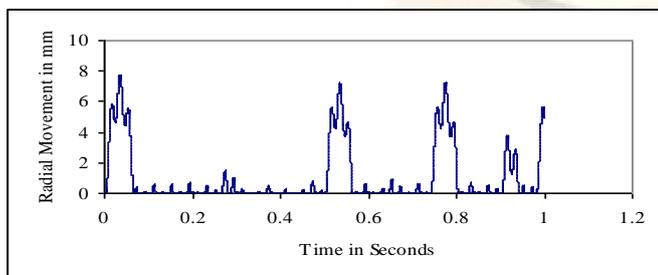
Fig.9 Cu particle radial movement for 220kV with analytical electric field
