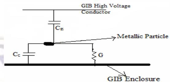
Fig.2 Circuit model of particle charging through the dielectric coating.
