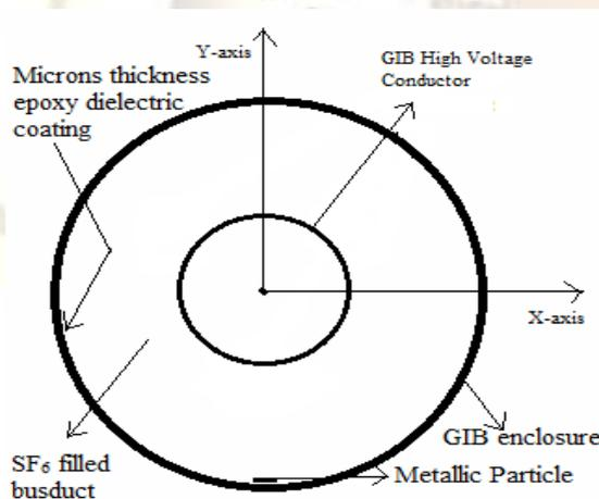
Fig.1 Typical single phase dielectric coated Gas Insulated Busduct
