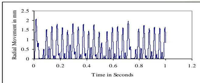
Fig.6 Cu particle radial movement for 100kV with image FEM electric field
