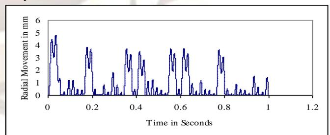
Fig.4 Al particle radial movement for 100kV with FEM electric field
