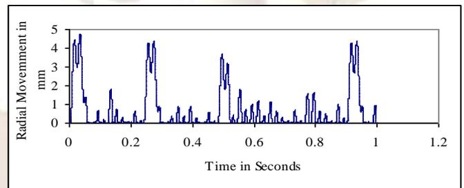
Fig.3 Al particle radial movement for 100kV with analytical electric field
