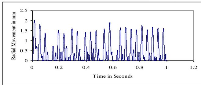
Fig. 5 Cu particle radial movement for 100kV with analytical electric field
