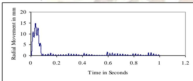
Fig.7 Al particle radial movement for 220kV with analytical electric field
