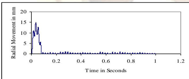
Fig.8 Al particle radial movement for 220kV with FEM electric field
