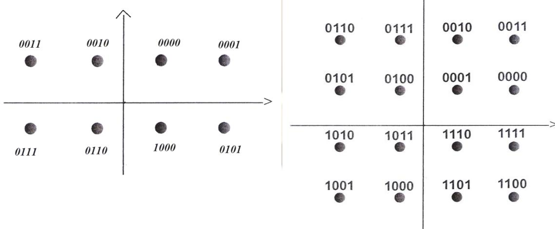
Figure-8QAM Constellation diagram
