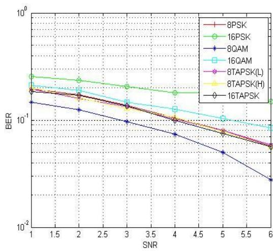
Figure1- Simulation results of non-coherent block codes at  $r=1$
