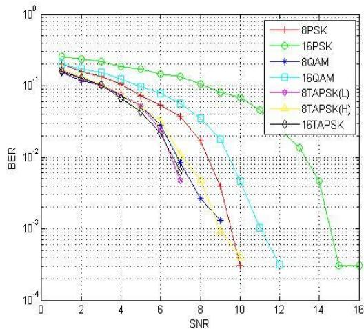
figure3- Simulation results of non-coherent block codes at  $d_{min}=4$
