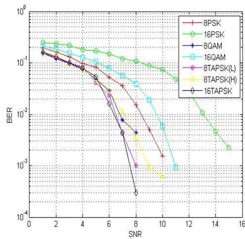
Figure2- Simulation results of non-coherent block codes at N=63
