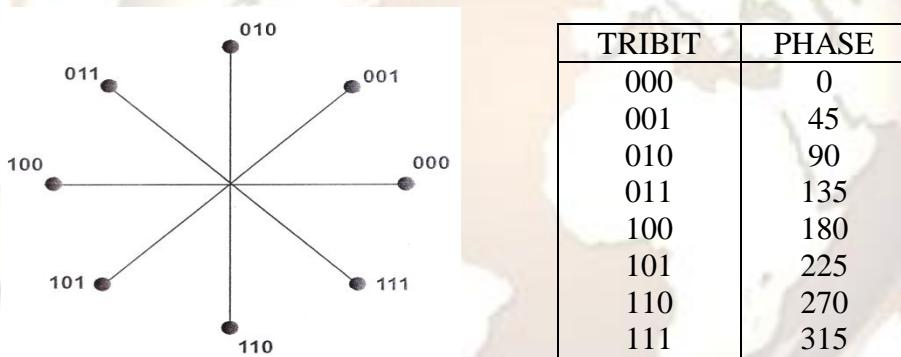
Figure 2. 8 PSK State constellation diagram
