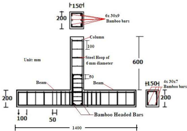
Figure 1. Dimensions of cross section areas.
