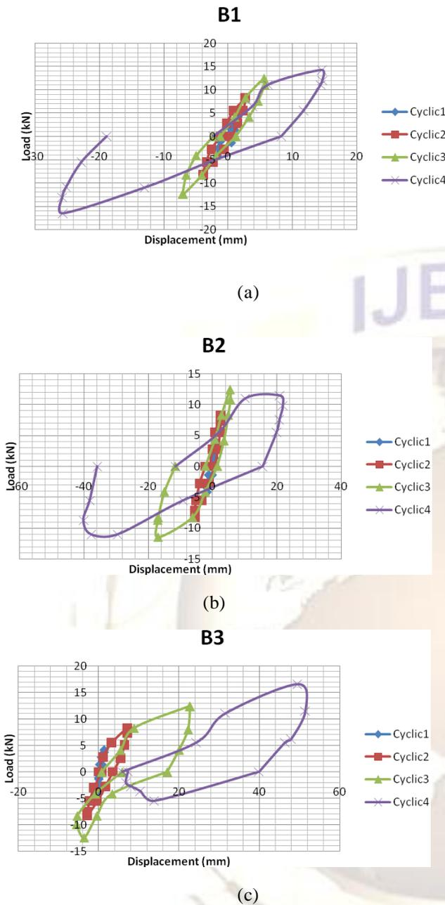
Figure 4. The relationship of test specimen load-displacement : (a) B1; (b) B2; (c) B3
