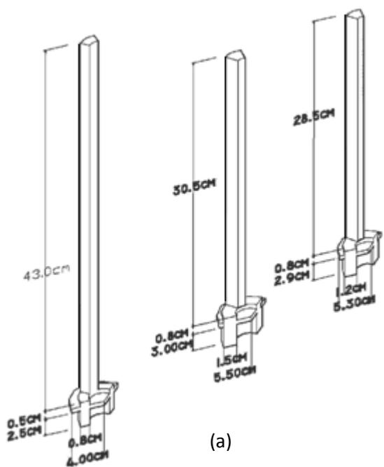
Figure 2. (a) Mechanical bamboo anchor B1, B2 and B3; (b) the position of the anchor.
