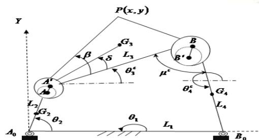
Fig.2. Schematic representation of a 4-bar mechanism with clearance
