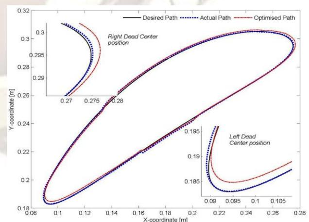
Fig. 6. Coupler curve for  $r_2=2$  mm and  $r_3=1$  mm
