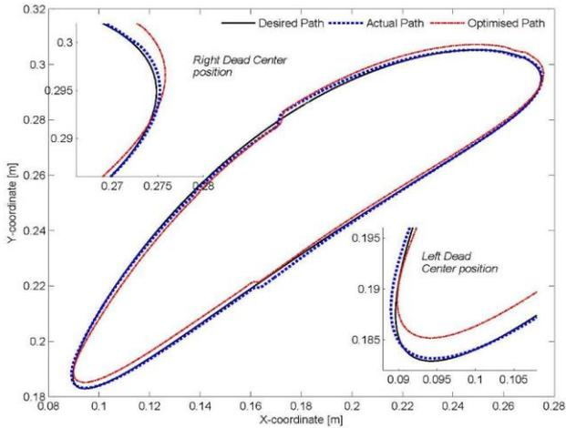
Fig. 7. Coupler curve for  $r_2=2$  mm and  $r_3=2$  mm
