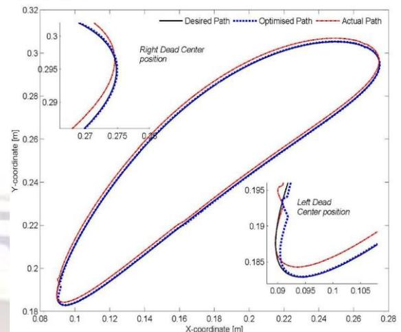
Fig. 4. Coupler curve for  $r_2=1$  mm and  $r_3=1$  mm
