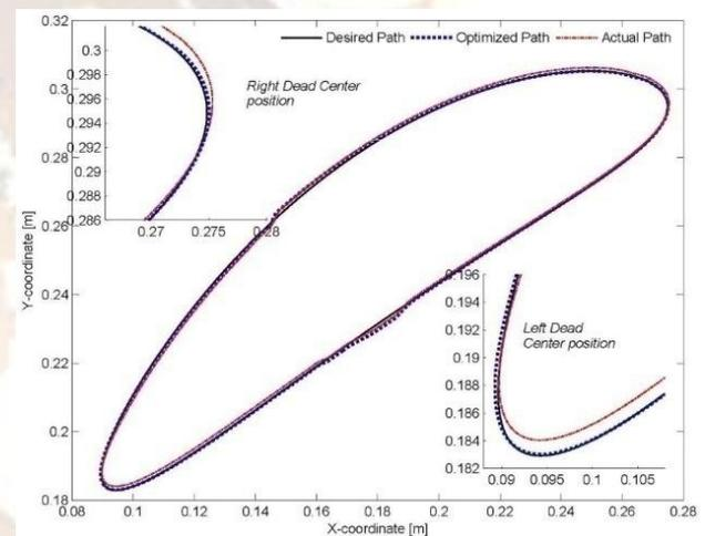
Fig. 5. Coupler curve for  $r_2=1$  mm and  $r_3=2$  mm
