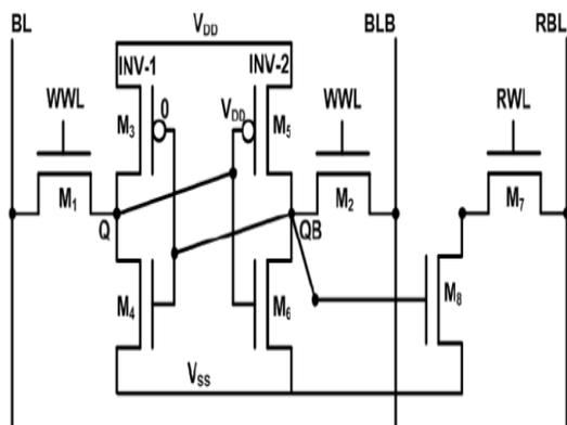
Figure 2: 8T SRAM cell
