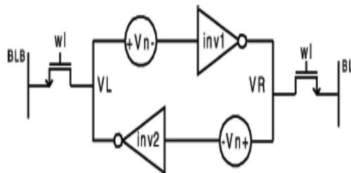
Figure 4: (a) The standard setup for the SNM definition.
