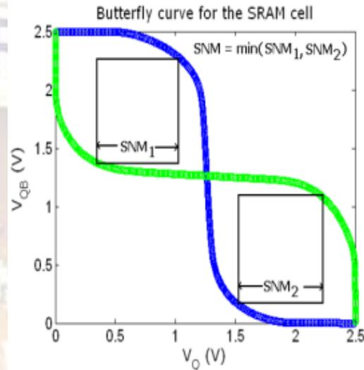
Figure 4: (b) Butterfly curve for the SRAM cell
