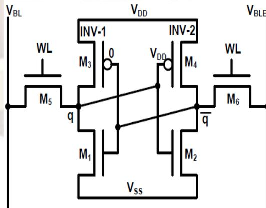
Figure 1: Standard 6T SRAM cell.
