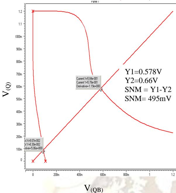
Figure 11: Simulation of WNM of 9T SRAM cell
