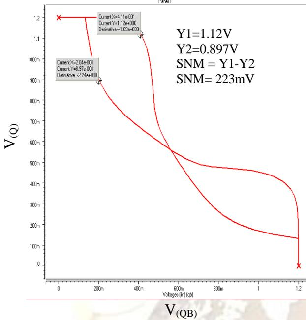
Figure 7: Simulation of RNM of 6T SRAM cell
