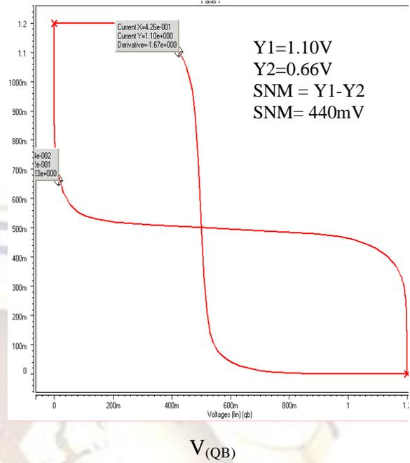
Figure 9: Simulation of RNM of 8T SRAM cell
