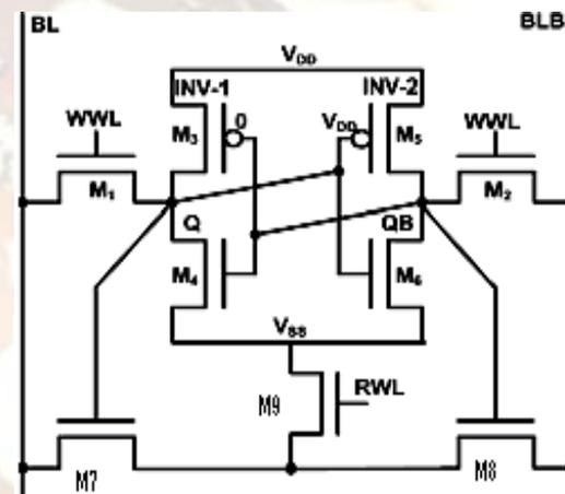
Figure 3: 9T SRAM cell.
