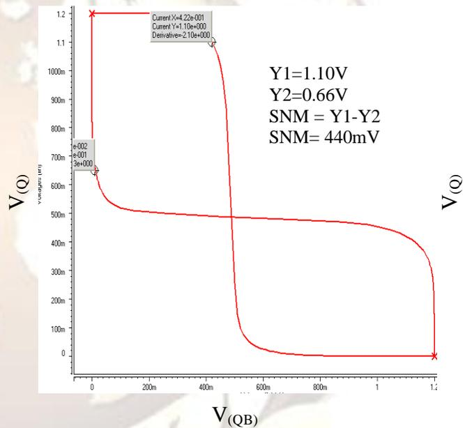
Figure 6: Simulation of HOLD SNM of 6T SRAM cell
