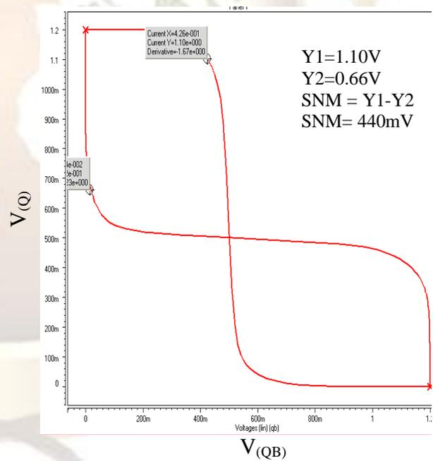
Figure 10: Simulation of RNM of 9T SRAM cell
