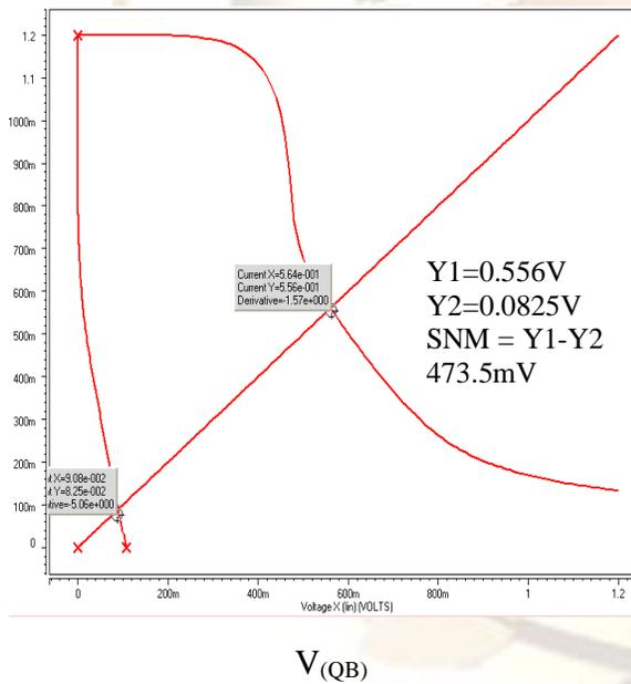
Figure 8: Simulation of WNM of 6T SRAM cell
