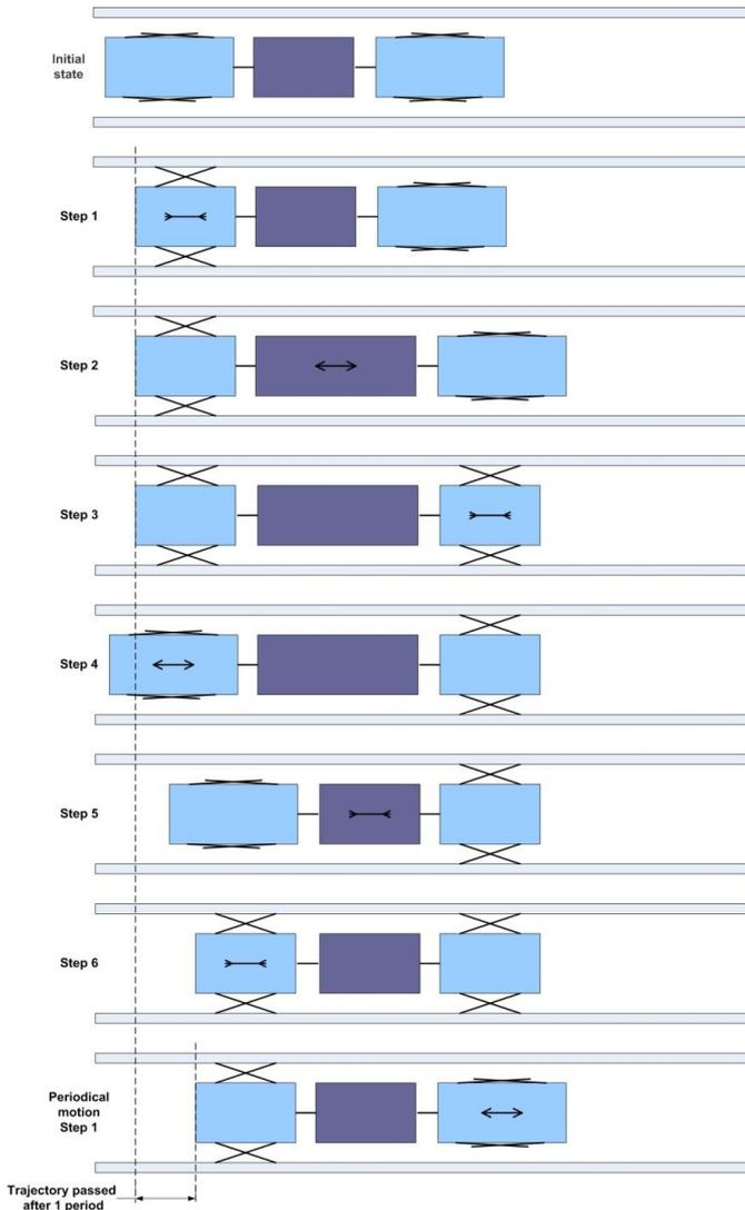
Fig. 2 Motion sequence of the minimachine
