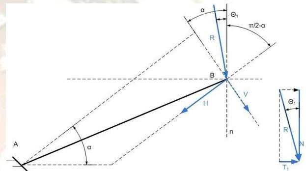
Fig. 5 Acting forces at forward motion.
