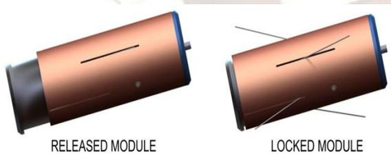
Fig. 3 Model of the front (back) in-pipe minimachine module
