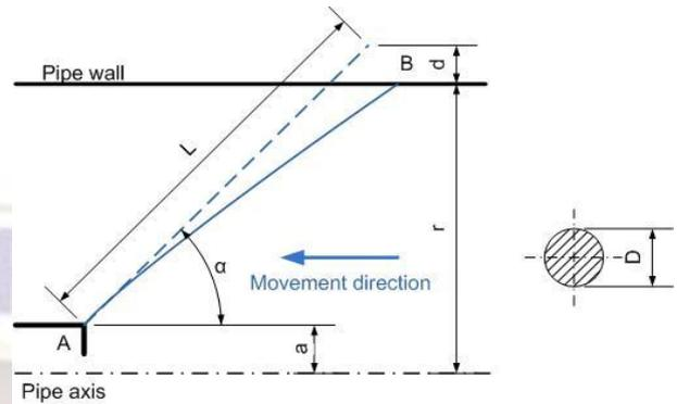
Fig. 4 Dimensions of minimachine bristle.
