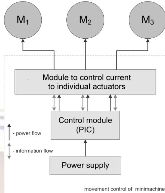
Fig. 7 Control scheme of the in-pipe minimachine
