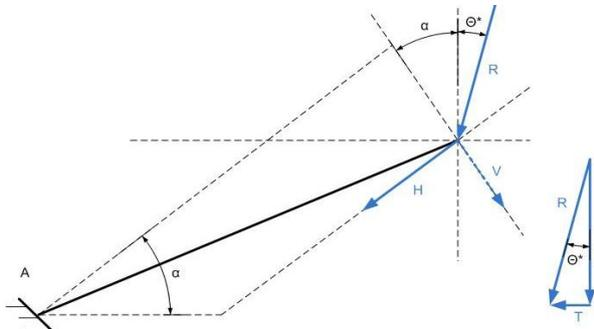
Fig. 6 Acting forces at bracing.
