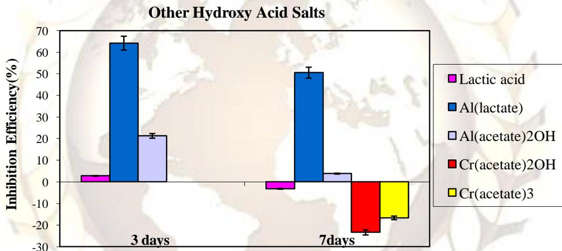
**Figure** Error! No text of specified style in document.-4 Inhibition Efficiency vs. Immersion Time Graph for  $\text{M}^{+n}(\text{X}^{-1})_{n-1}\text{OH}$  and  $\text{M}^{+n}(\text{X}^{-1})_n$  Type Hydroxy Acid Salts Other Than Gluconates
