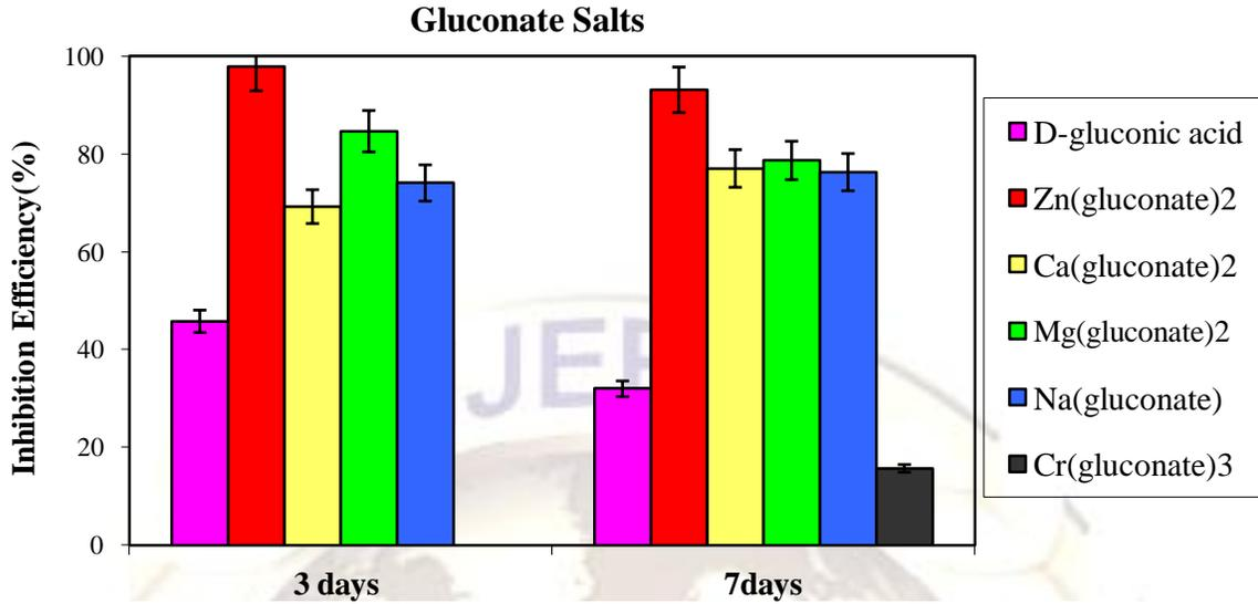
Figure Error! No text of specified style in document.-2 Inhibition Efficiency vs. Immersion Time Graph for  $M^{+n}(X^{-1})_n$  Type
