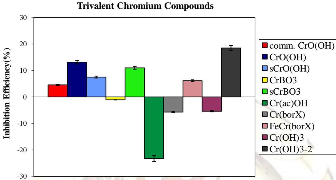
**Figure Error! No text of specified style in document.-10** Inhibition Efficiency Graph for Various
