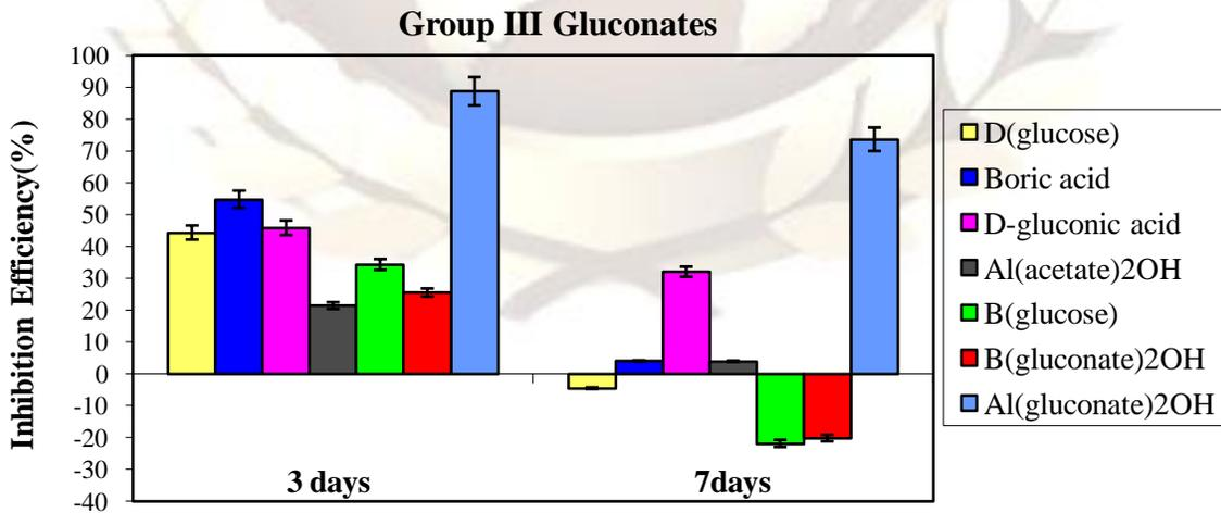
Figure Error! No text of specified style in document.-3 Inhibition Efficiency vs. Immersion Time Graph for  $M^{+n}(X^{-1})_{n-1}OH$  Type Gluconates
