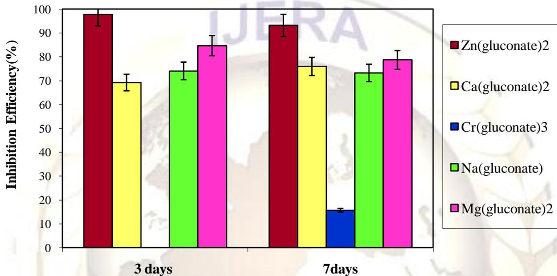
**Figure Error! No text of specified style in document.-12** Inhibition Efficiency vs. Immersion Time Graph for Formulations with Different Cationic Constituents
