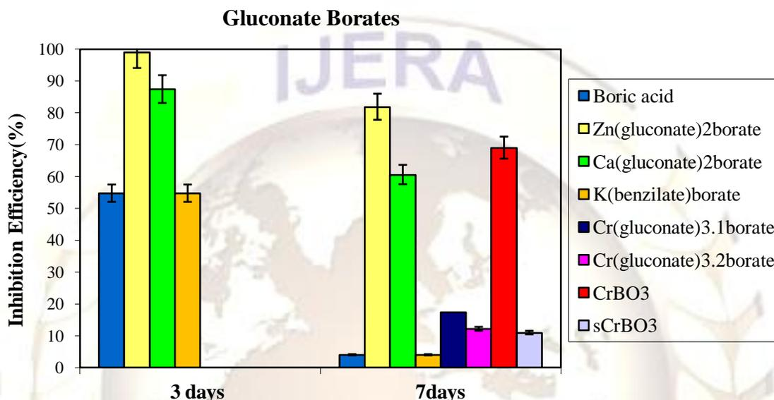
**Figure Error! No text of specified style in document.-7** Inhibition Efficiency vs. Immersion Time Graph for Boron Esters of Gluconate Salts and Their Derivatives
