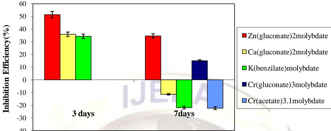
**Figure Error! No text of specified style in document.-5** Inhibition Efficiency vs. Immersion Time Graph for Molybdenum Esters of Gluconate Salts
