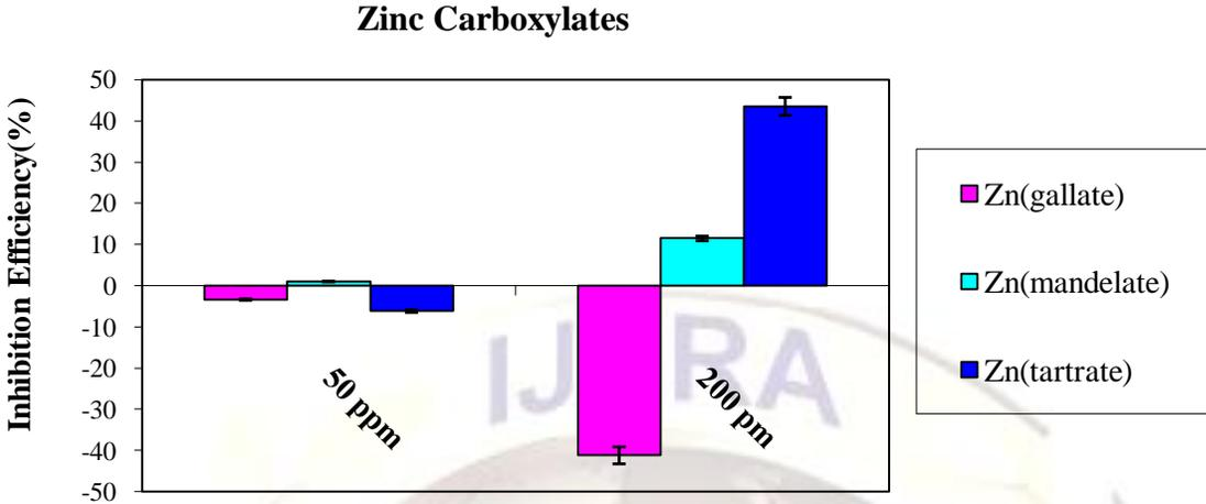
Figure Error! No text of specified style in document.-8 Inhibition Efficiency vs. Concentration Graph for Zinc Carboxylates
