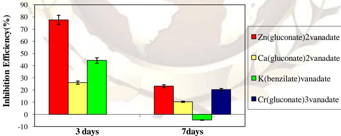
**Figure Error! No text of specified style in document.-6** Inhibition Efficiency vs. Immersion Time Graph for Vanadium Esters of Gluconate Salts
