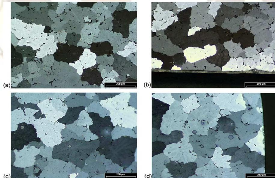
Fig. 10. Optical micrographs showing the original grains in different zones within the unprocessed billet.
