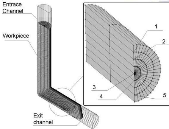
Fig. 2. ECAE process and considered zones within the billet, from reference [6].
