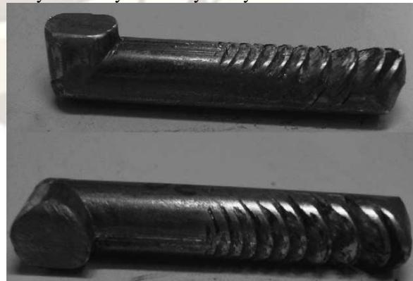
Fig. 1. Billets with cracks in the surface after  $N = 6$  ECAE passages.
