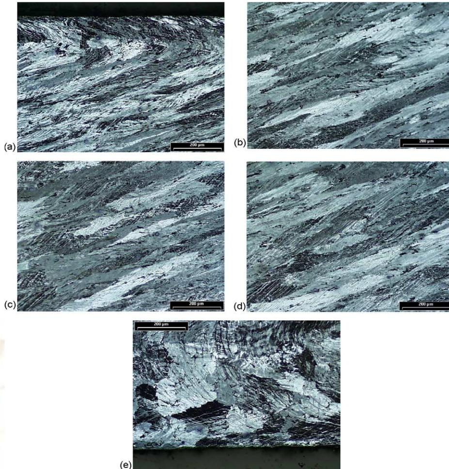
Fig. 11. Optical micrographs showing the deformed grains developed after three ECAE passages and route C, in different zones within the processed billet. (a) Zone 1 inner radius, (b) Zone 2, (c) Zone 3 central zone, (d) Zone 4 and (e) Zone (5) corresponding to the outer zone
