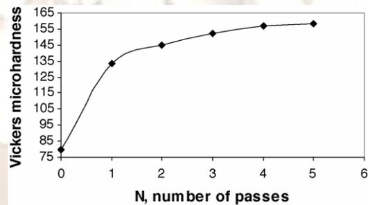
Fig. 13. Vickers microhardness vs. number of passes
