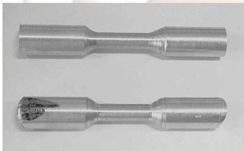
Fig. 3. Machined specimens for tensile test.
