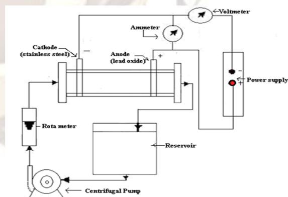
Fig.1: Schematic representation of Electrochemical Oxidation System
