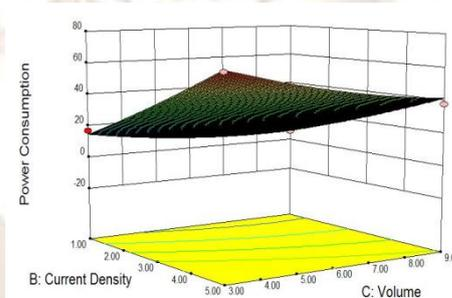
Fig 10: Current Density and Volume on Power consumption
