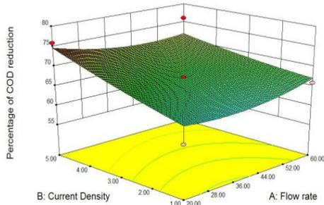
Fig 3: Flow Rate and Current Density on Percentage of COD Removal
