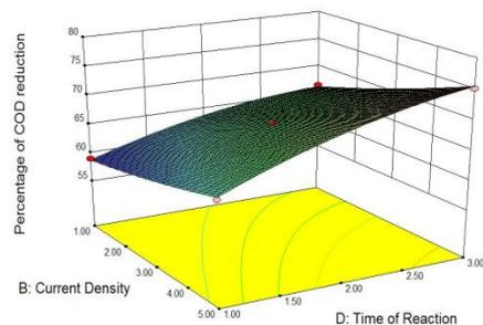
Fig 5: Current density and Time on Percentage of COD Removal
