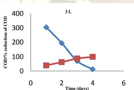
Fig 11: COD % reduction of COD on Time for 3 L volume electrolyte
