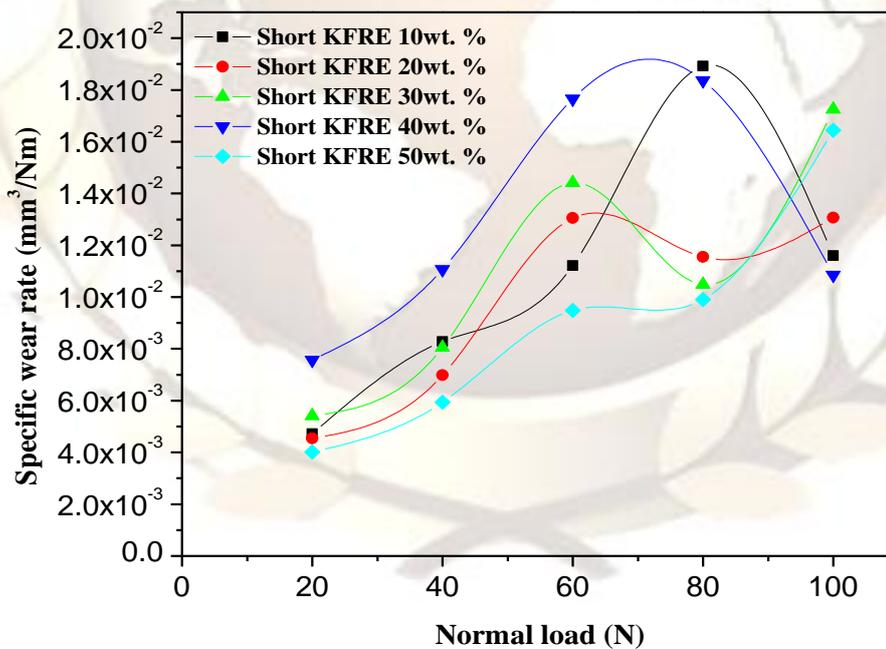
Fig. 7b Effect of normal load on specific wear rate of the short Kevlar fiber reinforced epoxy (KFRE) composites (At constant sliding velocity: 72cm/sec, sliding distance: 60m and abrasive size: 375 μm)
