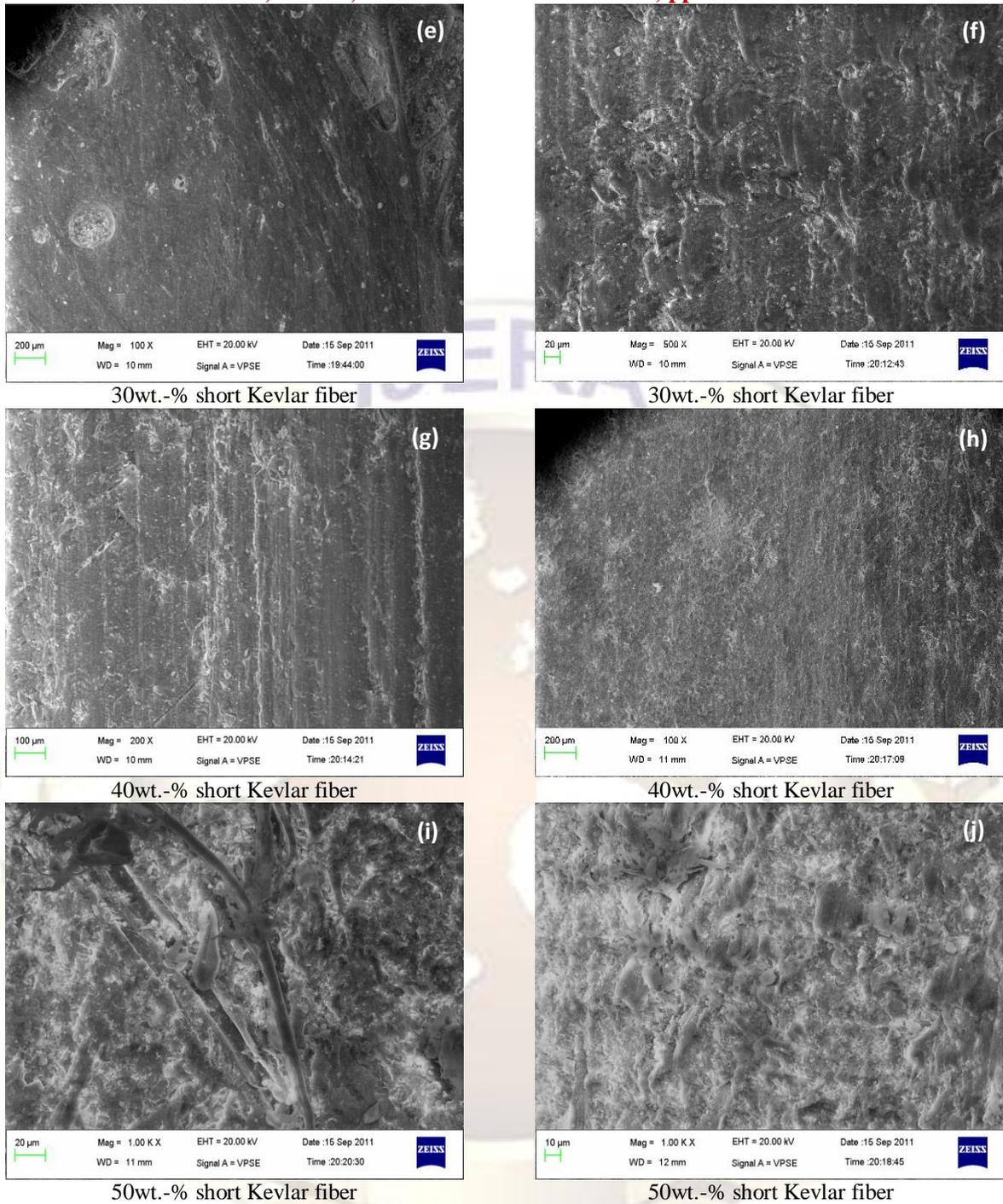
**Fig.10** SEM micrographs showing surface details of short Kevlar fiber reinforced epoxy composites
