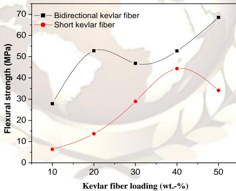
Fig. 3 Effect of fiber loading on flexural strength of Kevlar fiber reinforced epoxy composites
