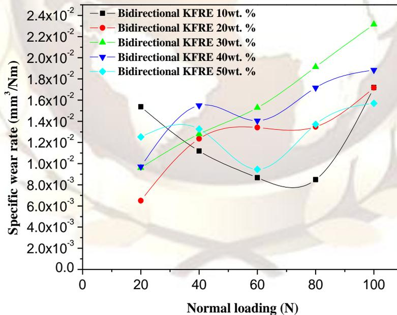
Fig. 6b Effect of normal load on specific wear rate of the bi-directional Kevlar fiber reinforced epoxy (KFRE) composites (At constant sliding velocity: 72cm/sec, sliding distance: 60m and abrasive size: 375  $\mu$ m)
