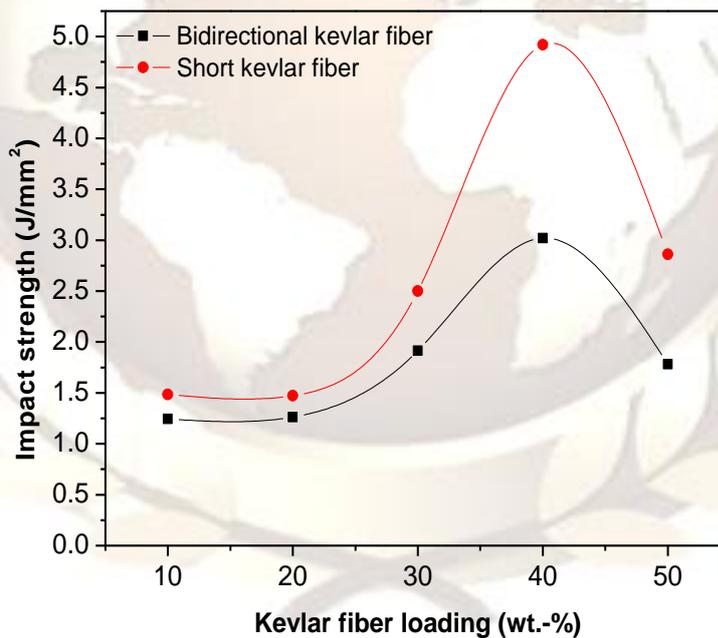
Fig. 5 Effect of fiber loading on impact strength of Kevlar fiber reinforced epoxy composites
