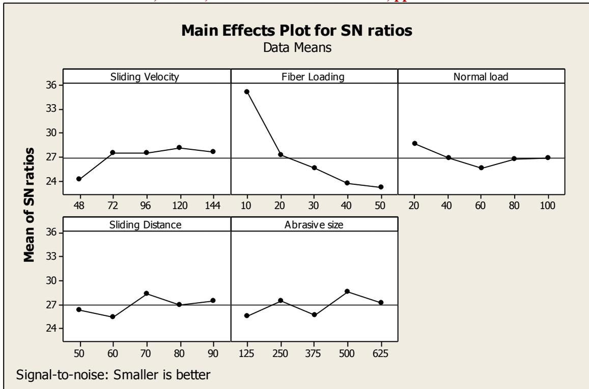
**Fig. 8a** Effect of control factors on signal-to-noise ratio of bi-directional Kevlar fiber reinforced epoxy composite
