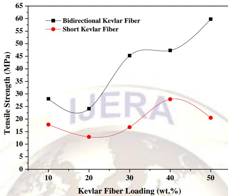
Fig. 2 Effect of fiber loading on tensile strength of Kevlar fiber reinforced epoxy composites
