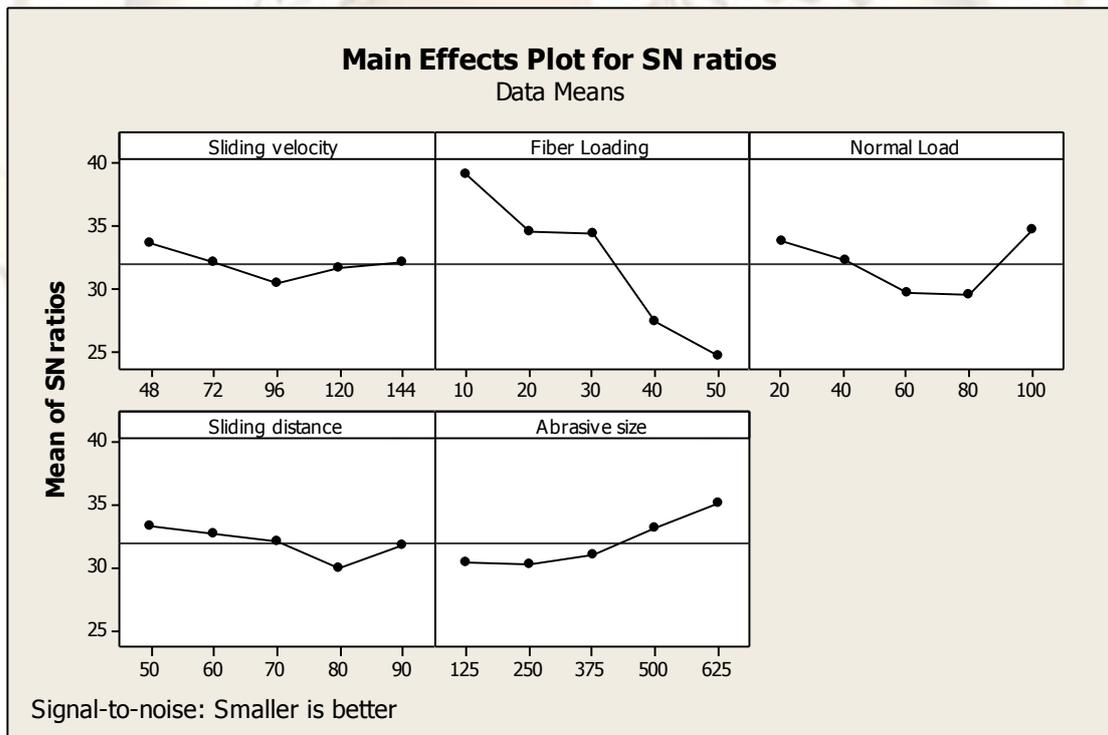
**Fig. 8b** Effect of control factors on signal-to-noise ratio of short Kevlar fiber reinforced epoxy composite
