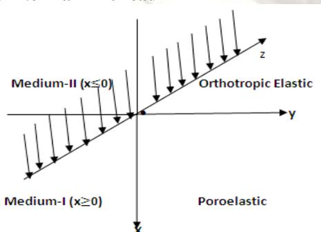
**Fig.1: A Normal line-load  $F_1$ , per unit length, acting in the positive x-direction on the interface  $x=0$  along z-axis.**
