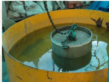
Fig. 3. Mould with saturation tank
