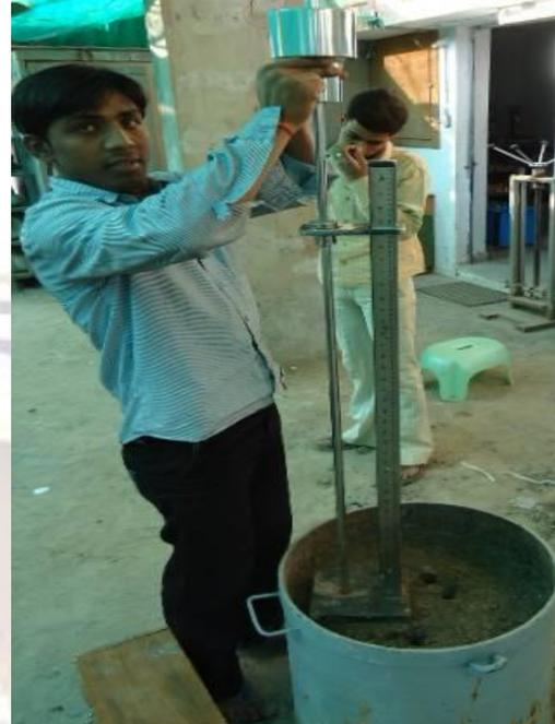
Fig. 5. Dynamic Cone Penetrometer
