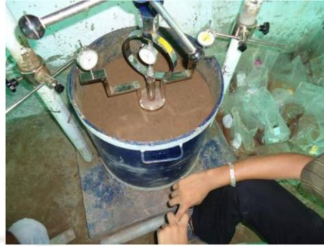
Fig. 2. The photograph of mould and Reaction frame
