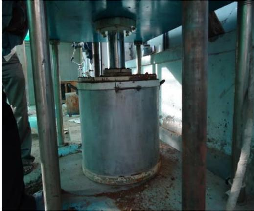
Fig. 4. Compression testing machine for static Compression of sample in mould
