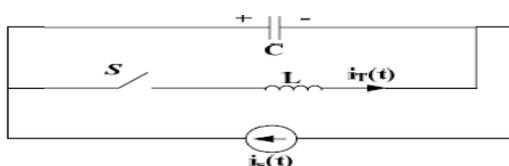
Fig. 2 A simplified TCSC circuit
