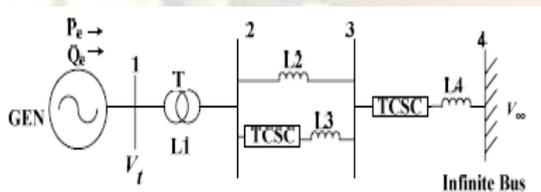
Fig:4 single machine infinite bus
