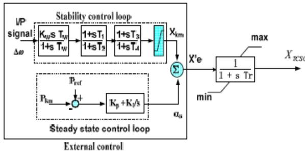
Fig. 3 shown below illustrate block diagram of TCSC model used in this paper for both operation modes
