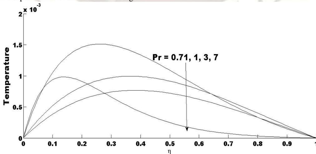
Figure 8. Temperature profiles for different values of  $Pr$ .
