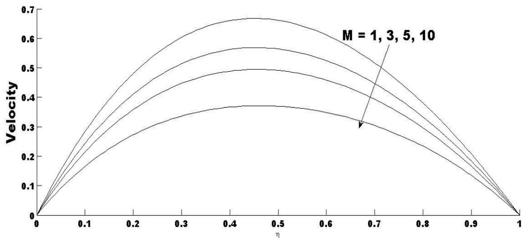
Figure 4. Velocity profiles for different values of M
