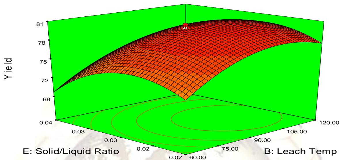
Figure 9: 3D plot of the effect of leaching temp and solid/liquid ratio on % yield.
