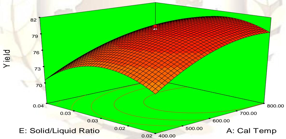
Figure 6: 3D plot of effect of calcination temp and solid/liquid ratio on % yield.
