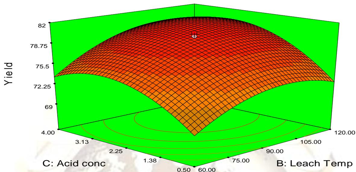
Figure 7: 3D plot of leaching temp and acid concentration on % yield.
