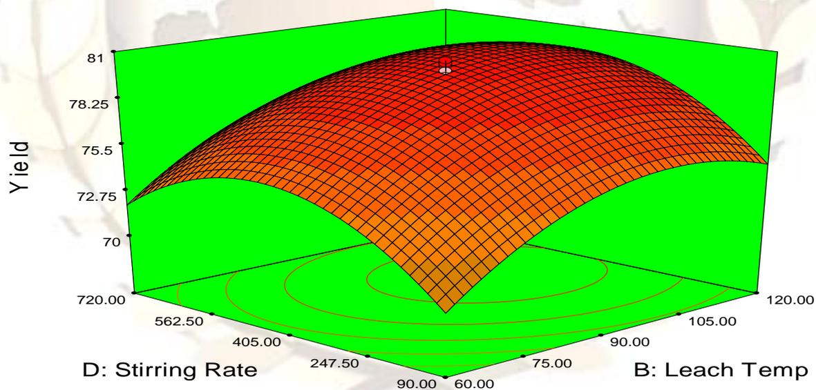
Figure 8: 3D plot of the effect of leaching temp and stirring rate on % yield.
