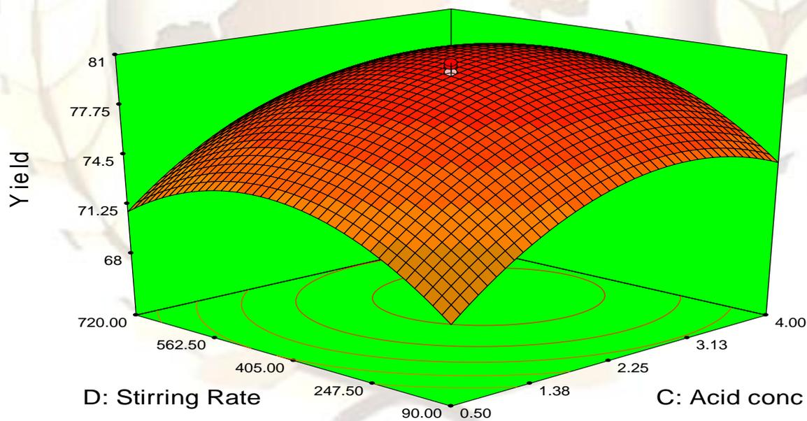
Figure 10: 3D plot of the effect of acid concentration and stirring rate on % yield.
