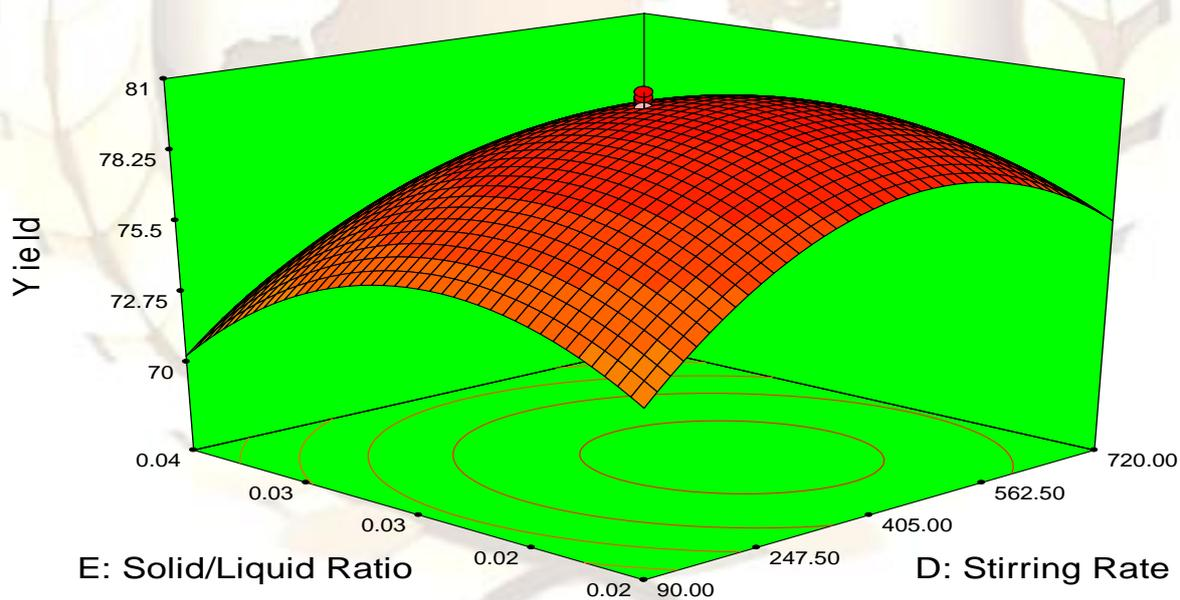
Figure 12: 3D plot of the effect of stirring rate and solid/liquid ratio on % yield.
