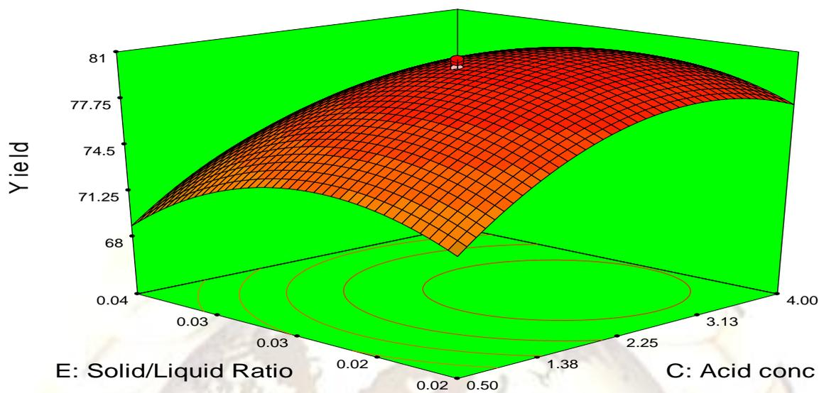
Figure 11: 3D plot of the effect of acid concentration and solid/liquid ratio on % yield.
