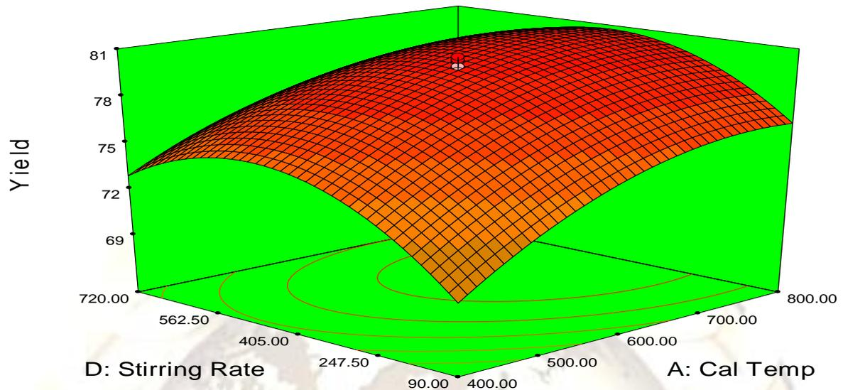
Figure 5: 3D plot of the effect of calcination temp and stirring rate on yield.
