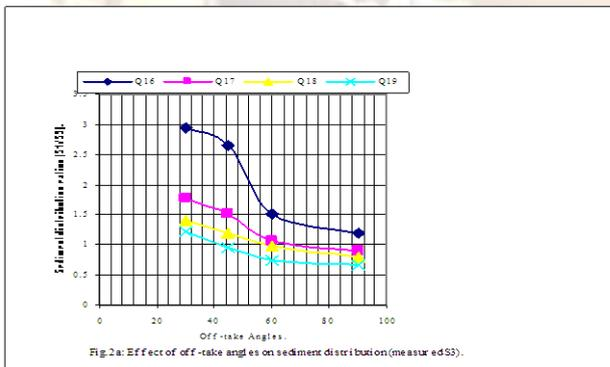
Fig.2a: Effect of off-take angles on sediment distribution (measured S3).
