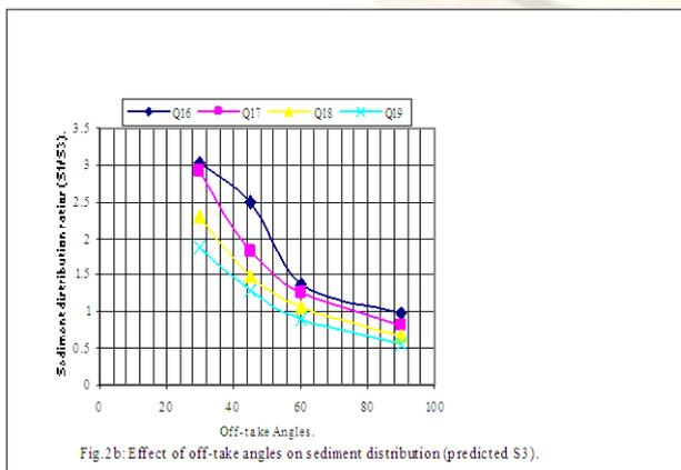
Fig.2b: Effect of off-take angles on sediment distribution (predicted S3).
