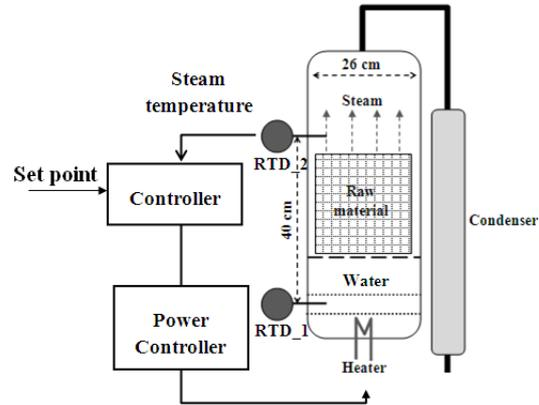
Fig.1 Schematic of a steam distillation process
