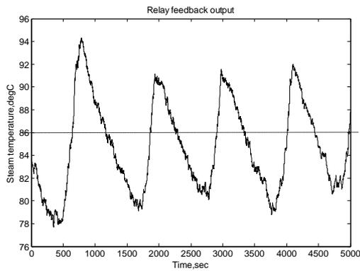
Fig. 5a Output from manual relay operation
