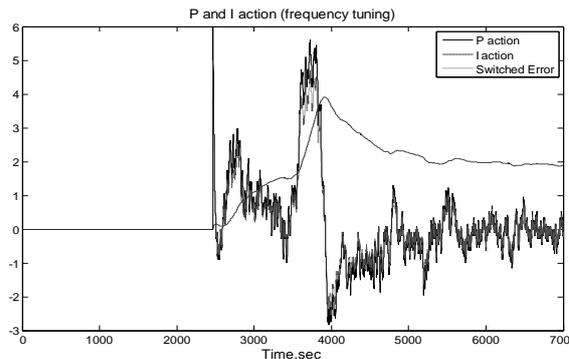
Fig. 7c P and I control signal with error switching
