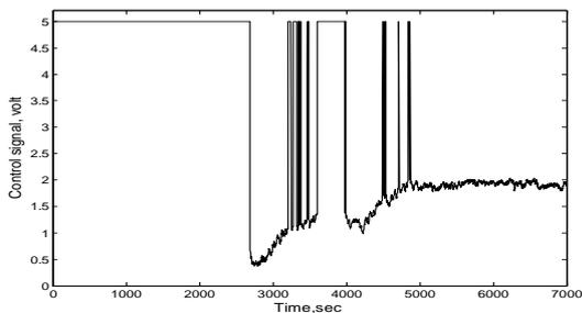
Fig. 6b PI control signal with reaction curve tuning
