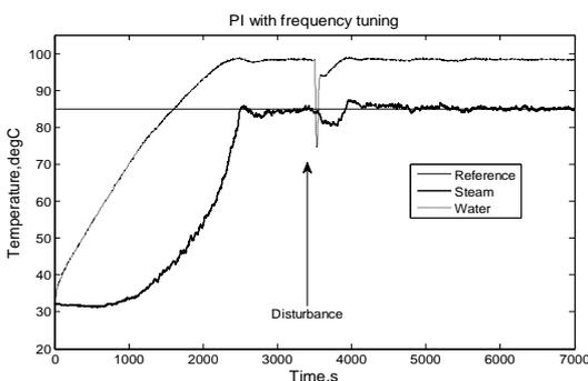
Fig. 7a Steam temperature with frequency tuning PI
