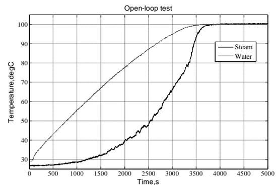
Fig.2 Open-loop response of steam and water temperature
