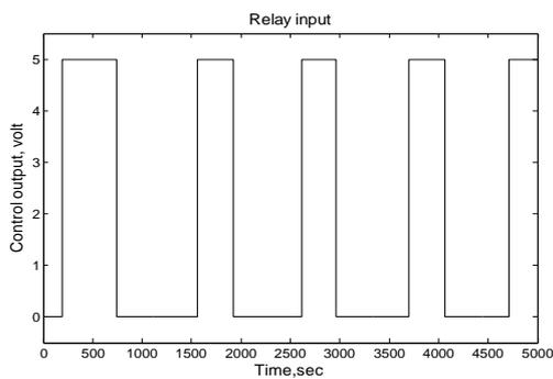
Fig. 5b Relay switching input signal
