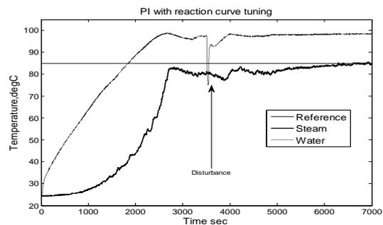
Fig. 6a Steam temperature with reaction curve tuning PI
