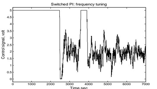
Fig. 7b PI control signal with frequency tuning
