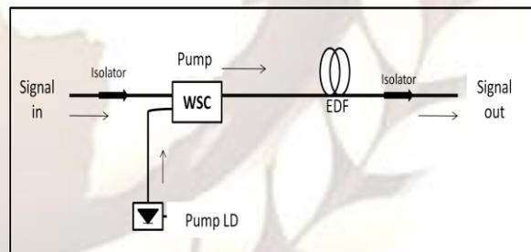
Fig.1 Forward pumped EDFA structure
