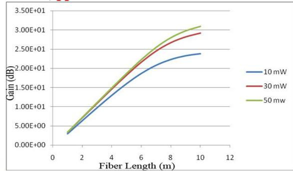
Fig.2 Gain variation for different pump powers
