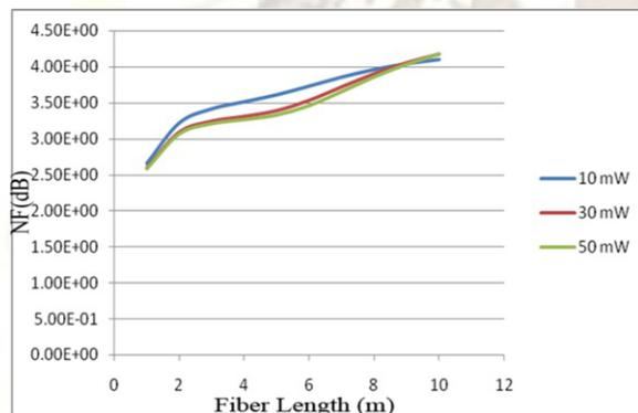
Fig.5 Noise Figure variation for different pump powers
