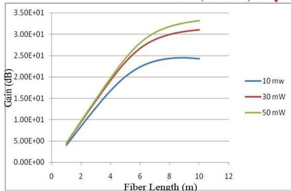
Fig.4 Gain variation for different pump powers
