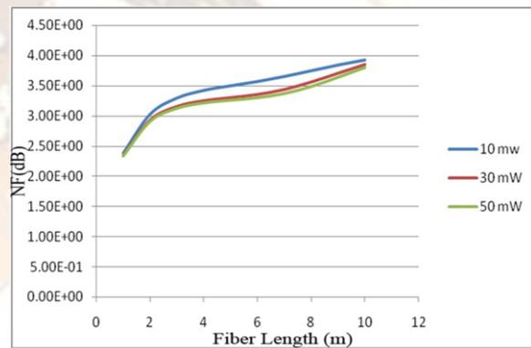
Fig.3 Noise Figure variation for different pump power
