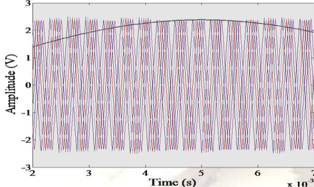
Fig.3: Reference and carrier waveforms for FFPSPWM technique
