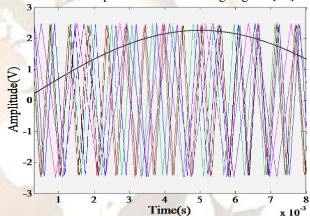
Fig.13: Reference and carrier waveforms of VFSPWM technique
