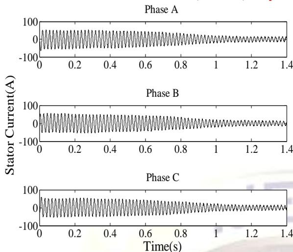
Fig.9: Stator current waveform of MLI with FFPSPWM
