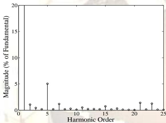
Fig.10: Frequency spectrum of stator current of MLI with FFPSPWM
