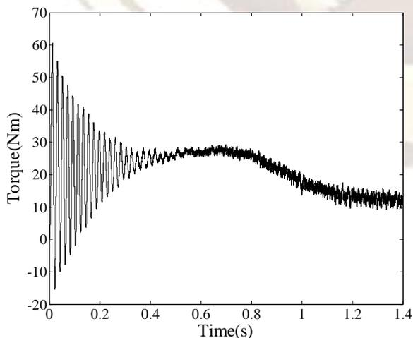
Fig.11: Torque vs. time characteristics of MLI with FFPSPWM
