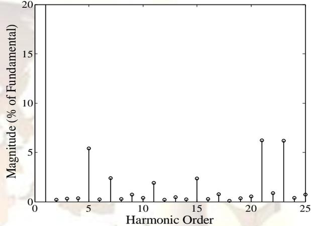
Fig.7: Frequency spectrum of phase voltage of asymmetric MLI with FFPSPWM
