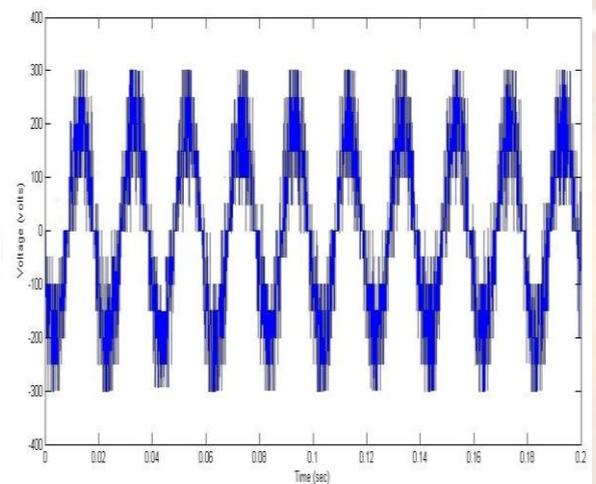
Fig.16: Line voltage (thirteen) of MLI with VFSPWM
