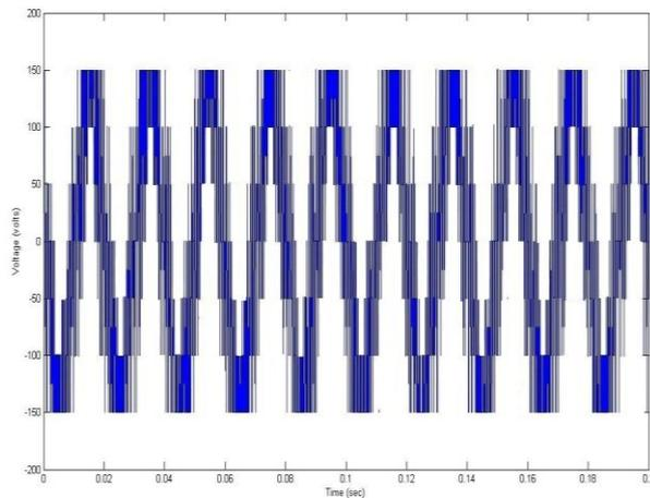
Fig.15: Phase voltage (seven) of asymmetric MLI with VFSPWM
