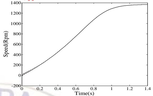
Fig.12: Speed vs. time characteristics of MLI with FFPSPWM
