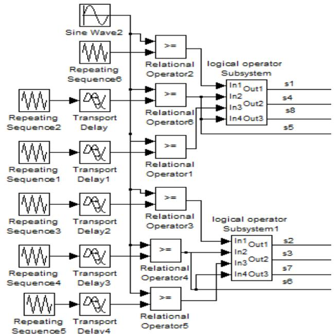
Fig.2: Circuit for carrier phase shifted PWM technique
