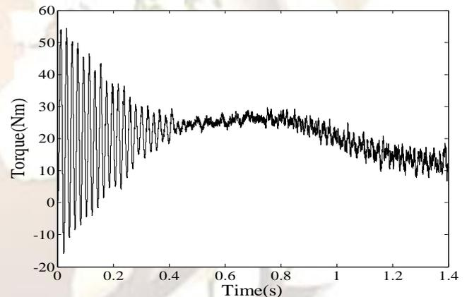
Fig.19: Torque vs. time characteristics of MLI with VFSPWM
