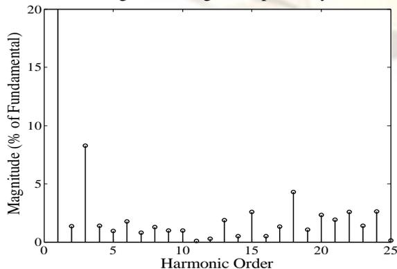
Fig.17: Frequency spectrum of phase voltage of MLI with VFSPWM
