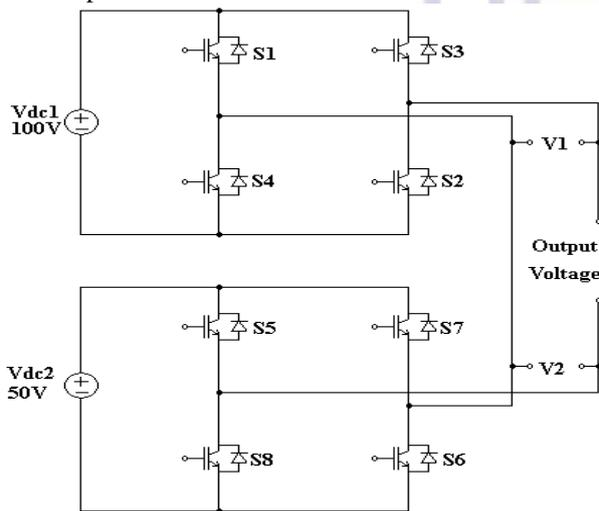
Fig.1: Proposed asymmetric cascaded MLI with three phase Induction motor load
