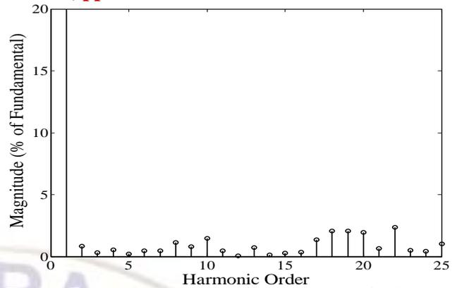
Fig.18: Frequency spectrum of line voltage of MLI with VFSPWM
