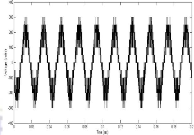
Fig.6: Line voltage (thirteen) of asymmetric MLI with FFPSPWM
