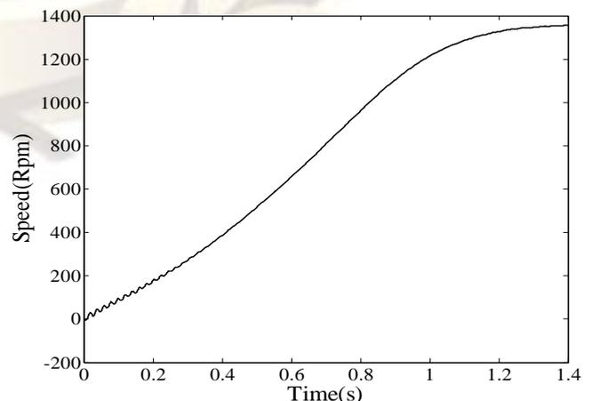
Fig.20: Speed vs. time characteristics of MLI with VFSPWM technique
