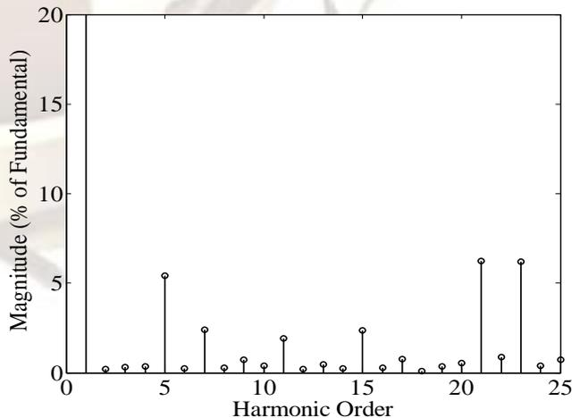
Fig.8: Frequency spectrum of line voltage of MLI with FFPSPWM
