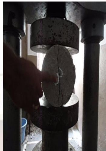
Fig. 3 Testing of Cylinder during split tensile strength test
