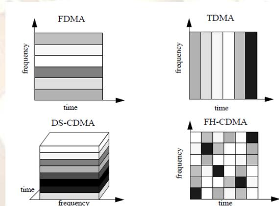
Figure 3: An illustration of various common multiple access protocols.
