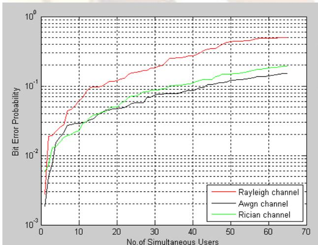
Figure 4: BEPs of the two-level FH-CDMA scheme versus the number of simultaneous users  $K$  over AWGN, and Rayleigh and Rician fading channels, where  $ML = 4$ ,  $ML \times ML = 4 \times 11$ ,  $ML \times ML = 11 \times 47$ ,  $ML = 13$ ,  $ML = 6$ , and  $ML/ML = 25$  dB.
