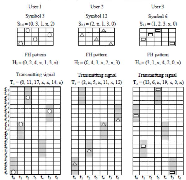
Figure 1: Example of the encoding process of the two-level FH-CDMA scheme with three simultaneous users. (The shaded columns in the transmitting signals,  $T_k$ , represent the frequency bands specified by the corresponding FH patterns,  $H_k$ , for  $k = \{1, 2, 3\}$ .)
