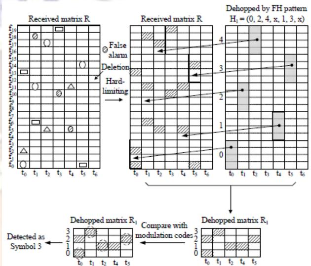
Figure 2: Example of the decoding and detection process of the two-level FH-CDMA scheme with user 1.
