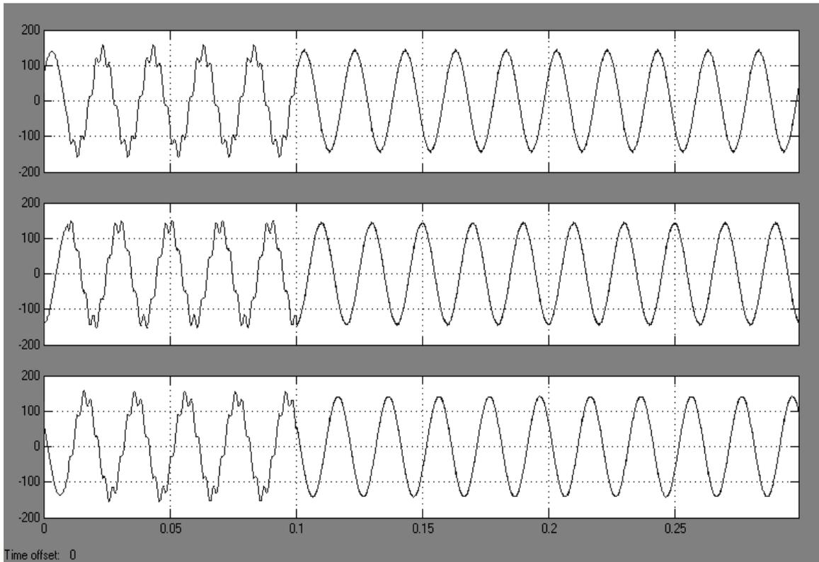
*Fig.8 Load voltage before and after compensation*
