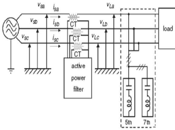
Fig.4 Circuit configuration for series active power filter
