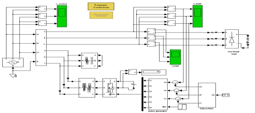
Fig.6 MATLAB model for Series active power filter
