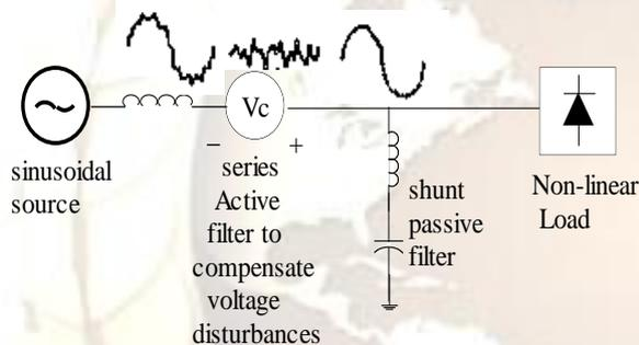
Fig.1 Filter voltage generation to compensate voltage disturbances
