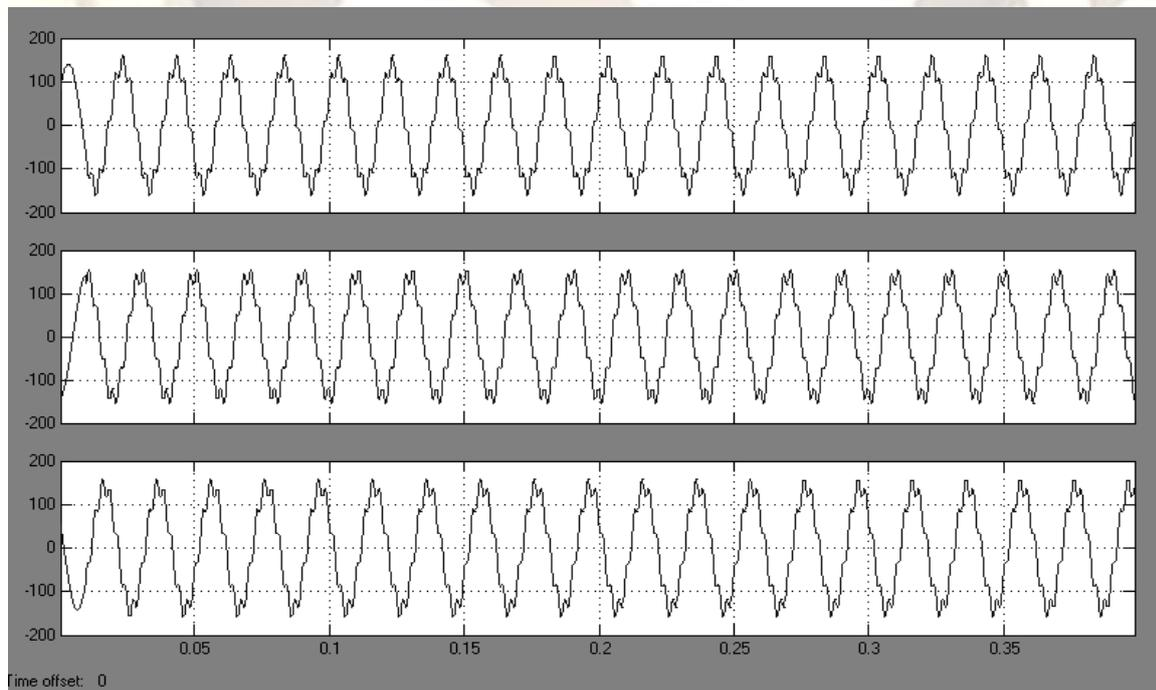
Fig.7 Source voltage containing harmonics
