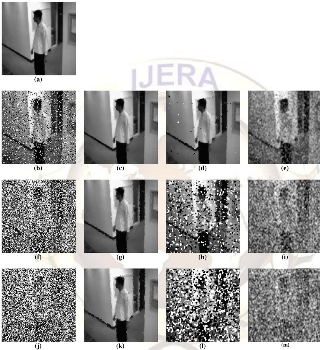
Fig. 4 Video Frames of vipmen.avi: (a) Original Frame; (b) at 20% noise density; (c) after Adaptive Median Filtering; (d) after Median Filtering; (e) After Mean Filtering; (f) at 60% noise density; (g) after Adaptive Median Filtering; (h) after Median Filtering; (i) After Mean Filtering; (j) at 75% noise density; (k) after Adaptive Median Filtering; (l) after Median Filtering; (m) After Mean Filtering.
