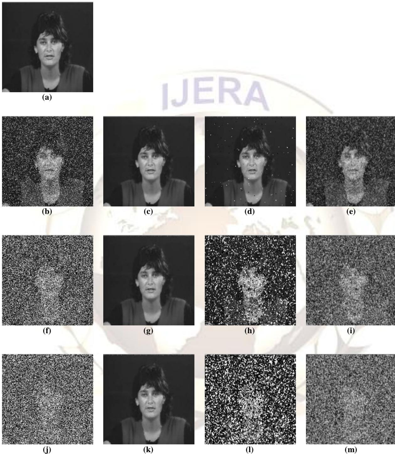
Fig. 3 Video Frames of miss\_america.avi: (a) Original Frame; (b) at 20% noise density; (c) after Adaptive Median Filtering; (d) after Median Filtering; (e) After Mean Filtering; (f) at 60% noise density; (g) after Adaptive Median Filtering; (h) after Median Filtering; (i) After Mean Filtering; (j) at 75% noise density; (k) after Adaptive Median Filtering; (l) after Median Filtering; (m) After Mean Filtering.
