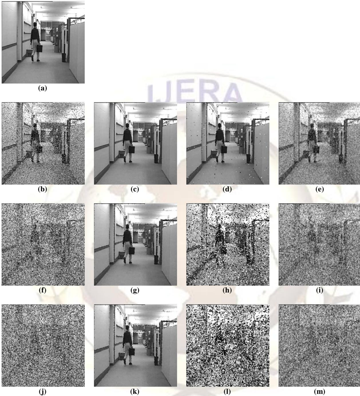
Fig. 5 Video Frames of Hall Monitor.avi: (a) Original Frame; (b) at 20% noise density; (c) after Adaptive Median Filtering; (d) after Median Filtering; (e) After Mean Filtering; (f) at 60% noise density; (g) after Adaptive Median Filtering; (h) after Median Filtering; (i) After Mean Filtering; (j) at 75% noise density; (k) after Adaptive Median Filtering; (l) after Median Filtering; (m) After Mean Filtering.
