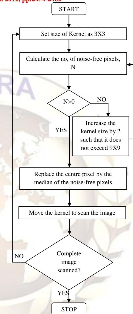
Fig. 2 Flowchart for Adaptive Median Filter
