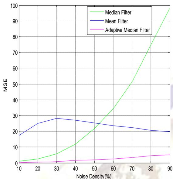
Fig.6 Plot of Mean Squared Error (MSE) vs. Noise Density (%)
