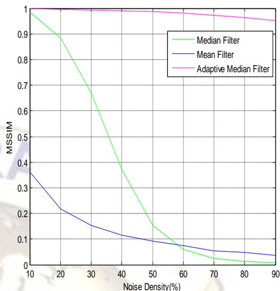
Fig. 8 Plot of Structural Similarity Index (MSSIM) vs. Noise Density (%)
