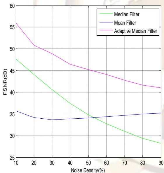
Fig. 7 Plot of Peak Signal to Noise Ratio (PSNR) in dB vs. Noise Density (%)
