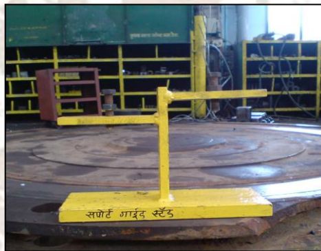
Photograph: Offline Height Setting of Jack
