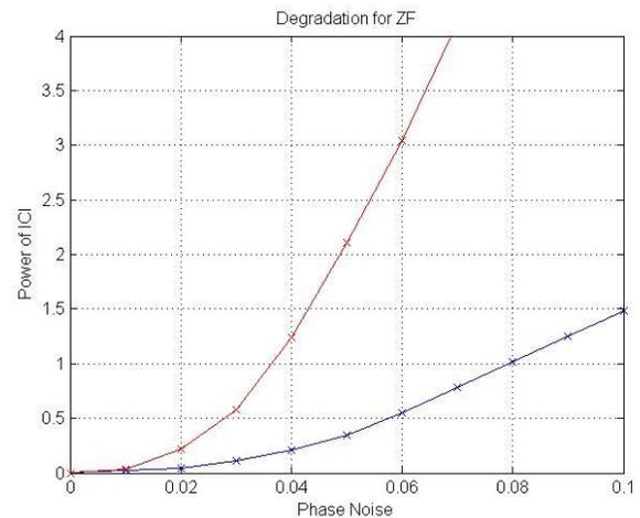
Fig.3. power of the ICI contribution for the ZF receiver with independent fading and ideal channel estimation. As the phase noise increases the ici also increases. The curves of the ICI power vs.  $B$  show a very good matching, although the first order approximation of is slightly optimistic
