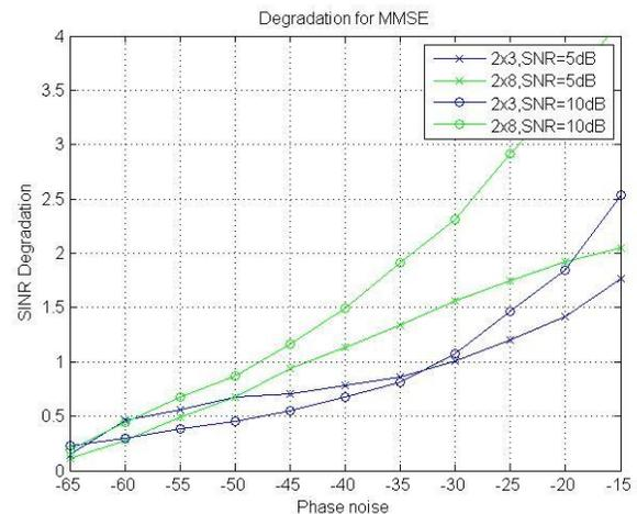
Fig.4.degradation for MMSE as a function of the phase noise at  $0.1/T$ , with exponential  $T_{rms}=0.1t$ , estimation error  $MSE=-30db$  and refrence  $SNR=5db$  and  $SNR=10db$  as phase noise increase the SINR degradation more.
