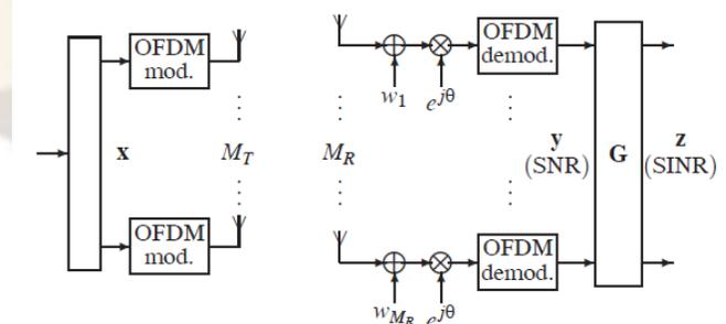
Fig1:Scheme of the MIMO-OFDM system
