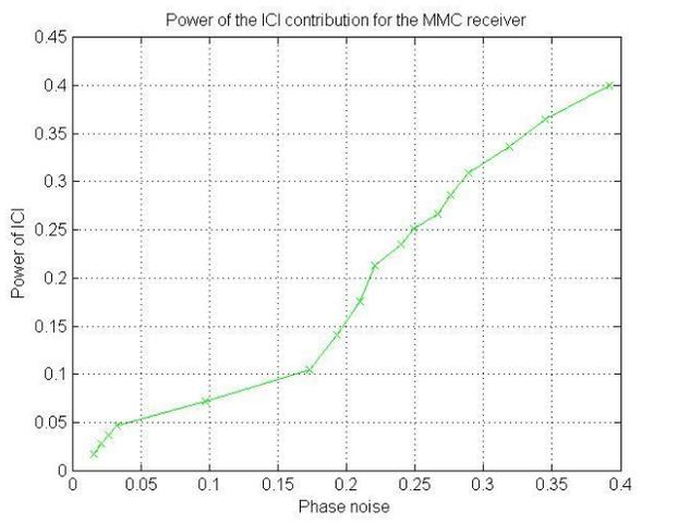
Fig.6.SINR degradation improves in ZF recovering that the phase noise increases power of ICI increases. When compared to the previous simulation results.
