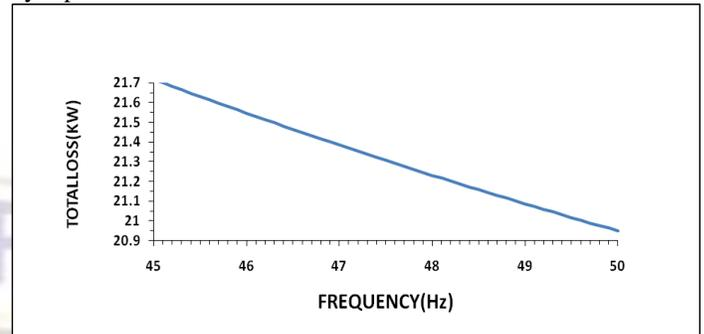
(Fig- 13 Frequency Vs Total loss)
