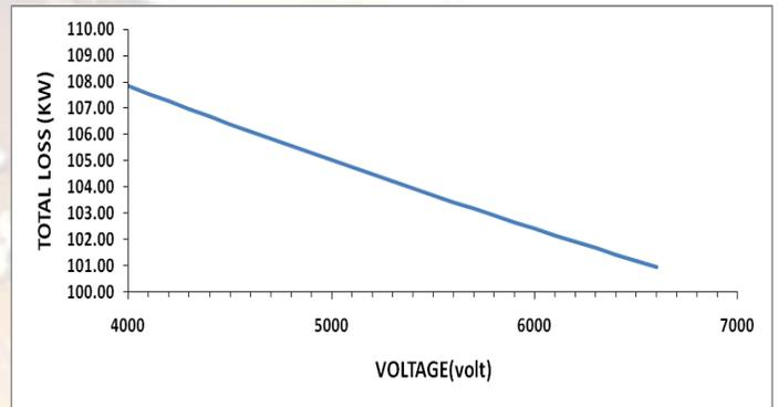
**(Fig- 7 Voltage Vs Total loss)**
