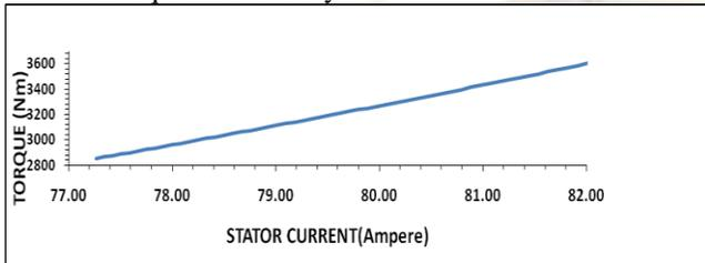
**Fig-4 Torque Vs Stator current**
