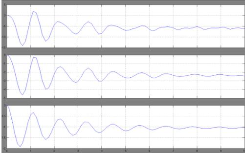
Figure 11 Rotor angle variations w.r.t time
