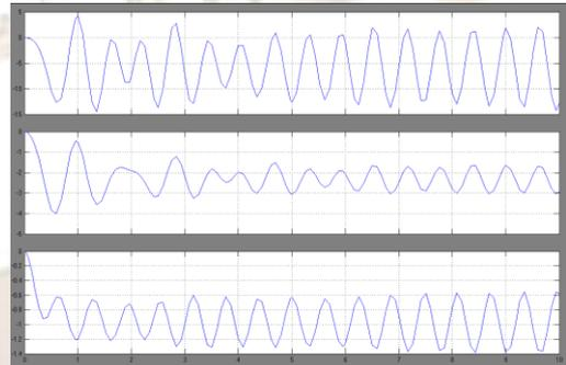
Figure 9 Rotor angle variations w.r.t time
