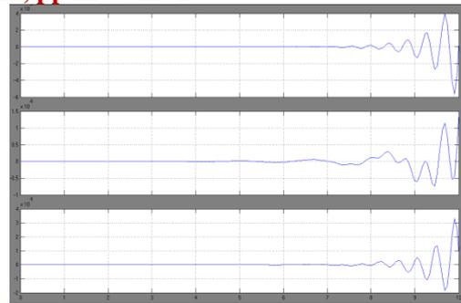
Fig 7 Rotor angle variations w.r.t time
