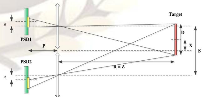
Fig. 1. Two 4Q-PSD and optic of them in the stereo mode.
