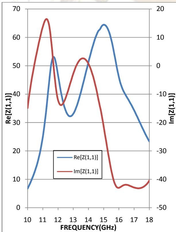
Figure 5. Input Impedance v/s frequency plot
