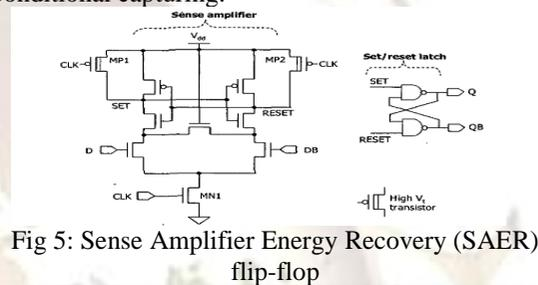
Fig 5: Sense Amplifier Energy Recovery (SAER) flip-flop
