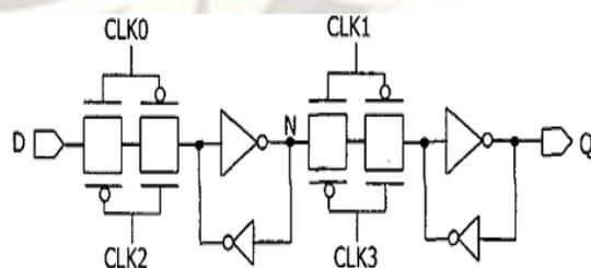
Fig 3: Conventional Four-Phase Transmission Gate(FPTG) energy recovery flip-flop
