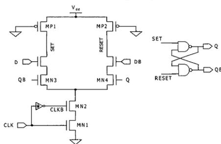
Fig 9: Differential Conditional Capturing Energy Recovery (DCCER) flip-flop
