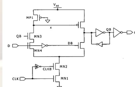
Fig.11: Single-ended Conditional Capturing Energy Recovery (SCCER) flip-flop
