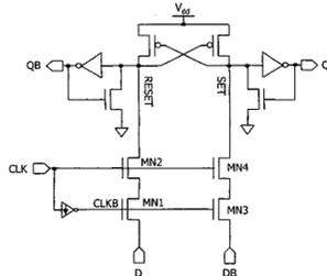
Fig 7: Static Differential Energy Recovery (SDER) flip-flop
