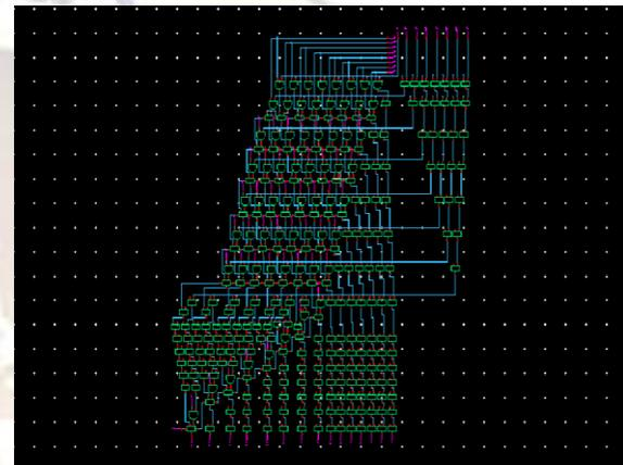
Fig 18: Pipelined array multiplier
