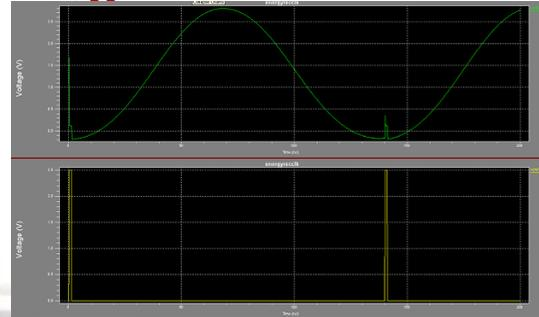
Fig 2: Output waveforms of generated energy recovery clock
