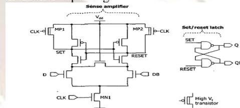
Fig 5: Sense Amplifier Energy Recovery (SAER) flip-flop
