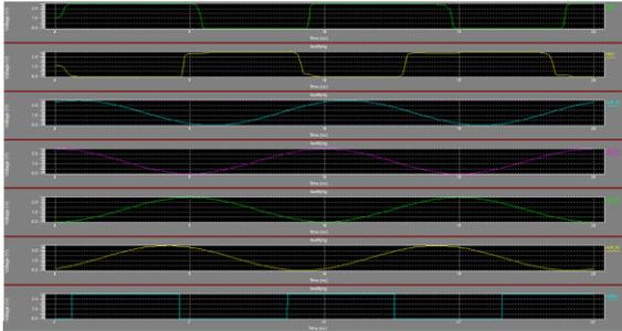
Fig 4: Output waveforms of FPTG flip-flop
