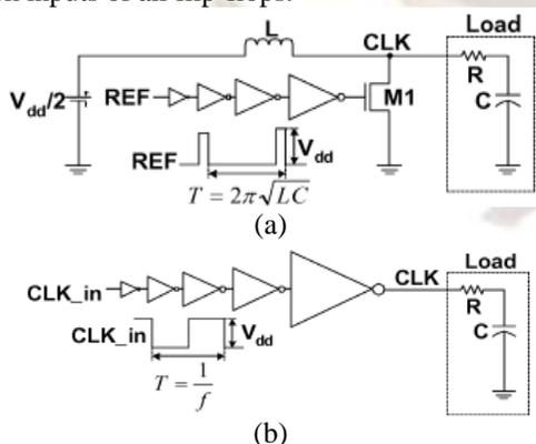
Fig 1(a): Resonant energy recovery clock generator
