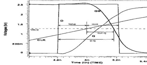
Fig 13: Sample waveforms illustrating timing definitions
