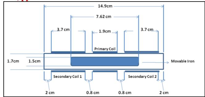
Fig.3. Modified LVDT connections with dimensions.
