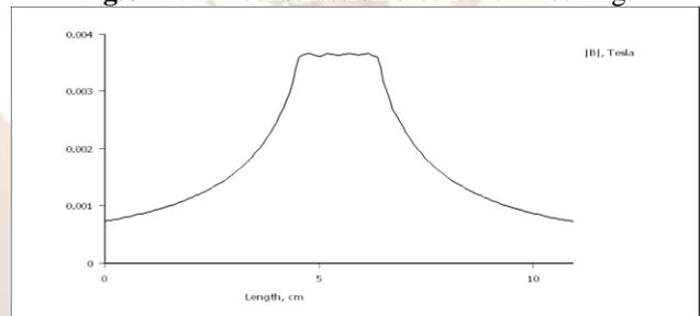
Fig.7. Distribution of flux density (B)
