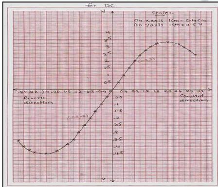
Fig.19. Variation of voltages in Modified LVDT.
