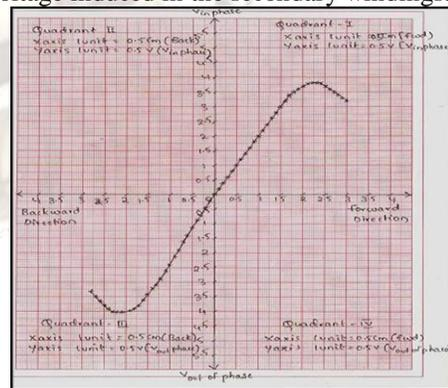
Fig.18. Variation of voltages in Conventional LVDT
