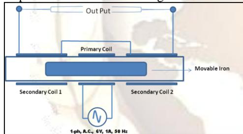
Fig.2. Modified LVDT with series connection of secondary windings.
