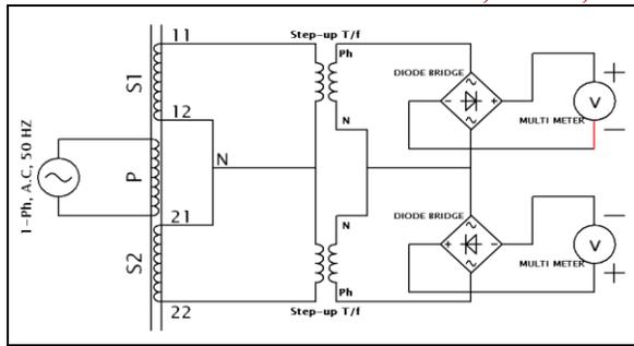
Fig.5. Modified LVDT working connections
