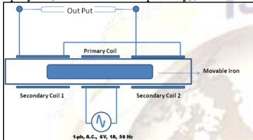
Fig.1. Conventional LVDT with back to back connection of secondary windings.
