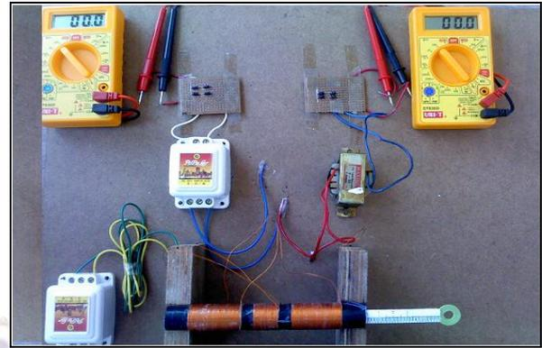
Fig.17. Real time working model of Modified LVDT
