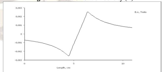
Fig.8. Distribution of normal flux density (B.n)
