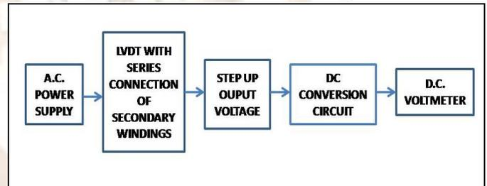
Fig.4. Block diagram shows the operation of Modified LVDT
