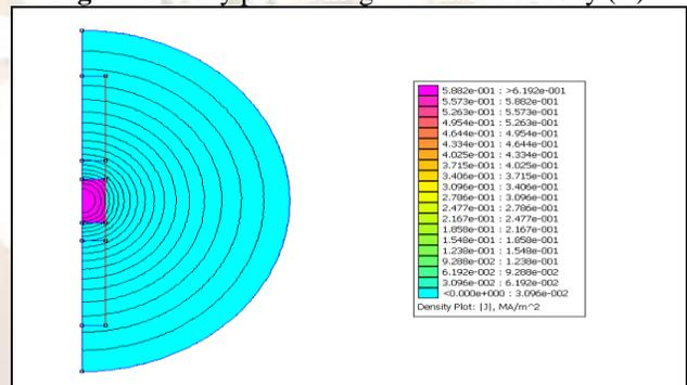
Fig.16. Density plot of current density (J)
