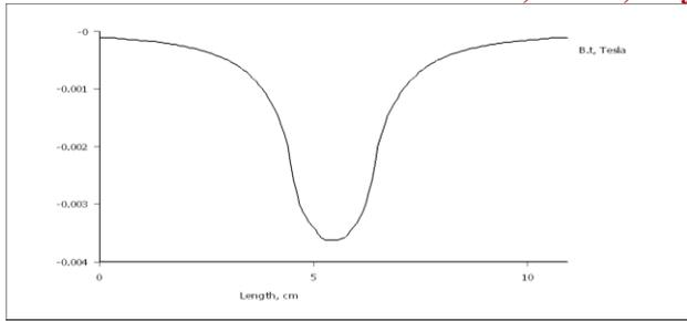
Fig.9. Distribution of tangential flux density (B.t)
