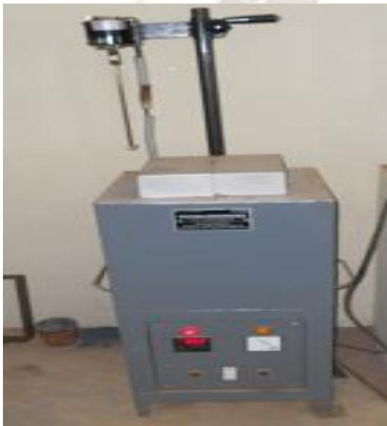
Fig. 1 stir casting equipment
