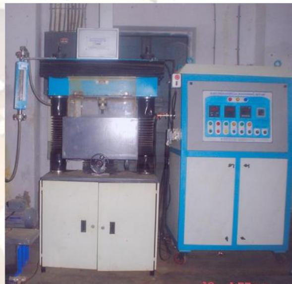
Fig. 2 Experimental setup of ECM
