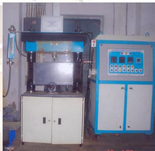
Fig. 2 Experimental setup of ECM
